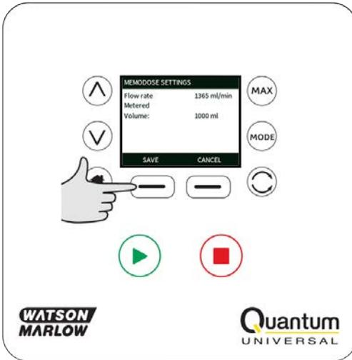
When MemoDose SETTINGS are complete the following screen is displayed; press **MEMODOSE** to start in MemoDose Mode or **BACK** to return to MemoDose settings.
