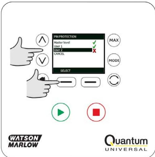
**ENABLE** user 2 security settings displays the PIN entry screen for User 2. To define a four digit User 2 PIN, use the  $\wedge$  /  $\vee$  keys to select each digit from 0-9. Once you have the required digit press the **NEXT DIGIT** key. After selecting the fourth digit press **ENTER**.
