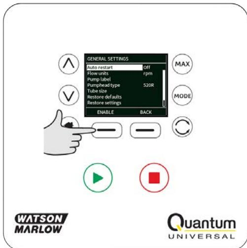
Use the  $\wedge$  /  $\vee$  keys to move the selection bar over **Pumphead** and press **SELECT**.
