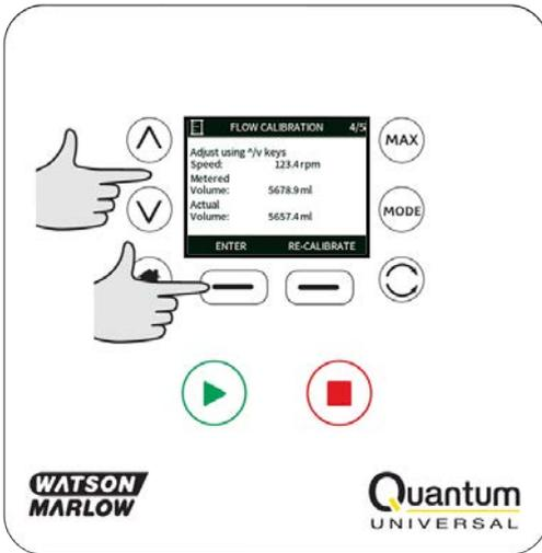
To accept the new calibration press **ACCEPT** or **RE-CALIBRATE** to repeat the procedure. Press **HOME** or **MODE** to abort.
