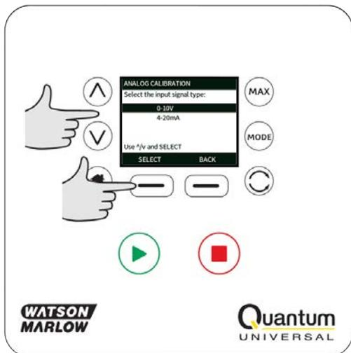
The pump gives the option to enter the high and low mA or V signals manually or via the analog input. Entering mA values is described here, however the process for entering V signals is identical.
