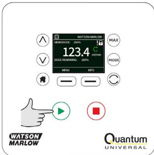
If the delivered dose differs from the volume required, the percentage may be adjusted within the limits 1% to 999% of the master dose. Use the ∧ / ∨ keys to alter the percentage. The new dose size is displayed as a percentage on the home screen.
