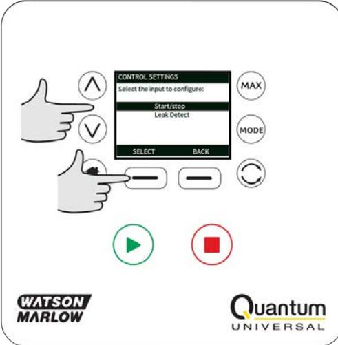
Use the  $\wedge$ / $\vee$  keys and press **SELECT** to choose the logic state of the chosen output.
