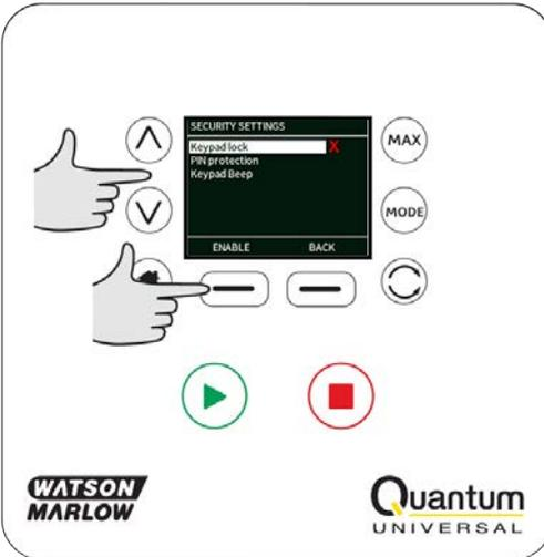
Once locked it will display the screen below when any key is pressed. To unlock the keypad press the two **UNLOCK** keys together.
