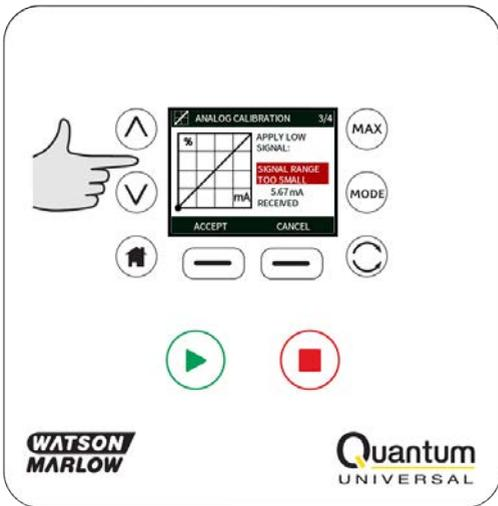
ACCEPT appears when low mA signal is within tolerance limits. Press **ACCEPT** to accept the low signal input or **CANCEL** to return to the previous screen.
