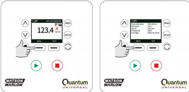
This will display the main menu as shown below. Use the  $\wedge$  /  $\vee$  keys to move the selection bar between the available options.
