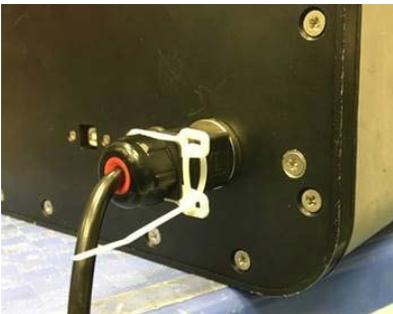
Ensure the security clip is secured to the power connector with a tie wrap (as shown) and the Harting power connector is in place before power is applied to the unit.
