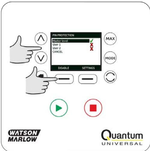
**ENABLE** user 1 security settings displays the PIN entry screen for User 1. To define a four digit User 1 PIN, use the  $\wedge$  /  $\vee$  keys to select each digit from 0-9. Once you have the required digit press the **NEXT DIGIT** key. After selecting the fourth digit press **ENTER**.
