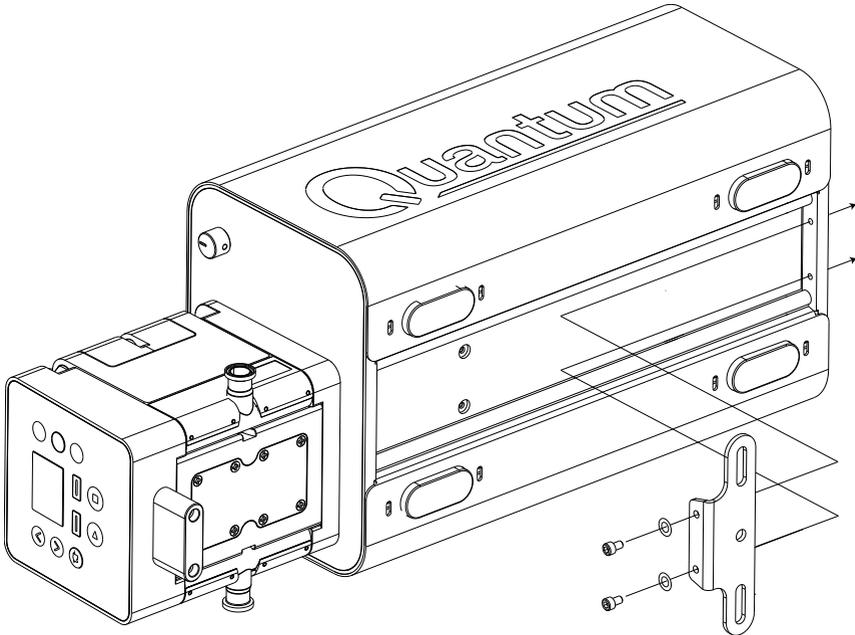
Secure the bolt down bracket to the pump body's mounting surface using 2xM10 bolts and M10 anti-vibration washers. M10 bolts and M10 washers are not supplied.
