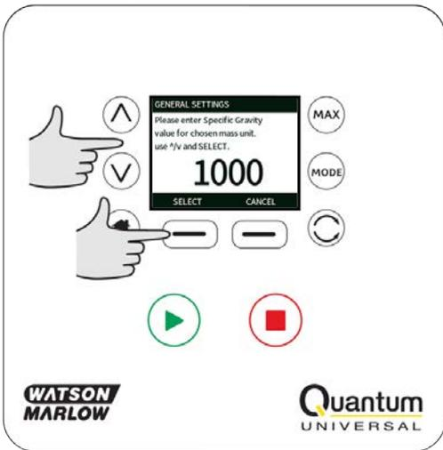
Use the  $\wedge$  /  $\vee$  keys to enter the value of the specific gravity, and press **SELECT**.
