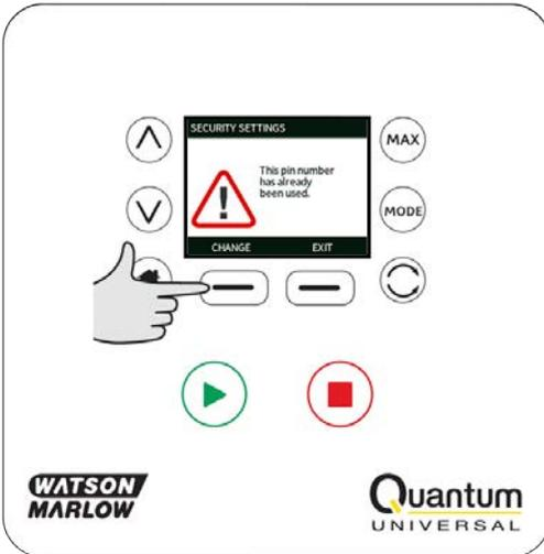
If the PIN entered does not allow access to the functionality the following screen will be displayed.
