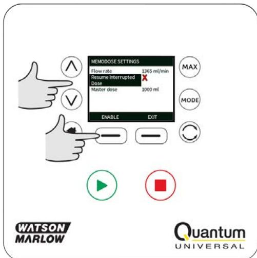
If resume interrupted doses has been set the following warning screen is displayed, press **CONFIRM** to save this setting.
