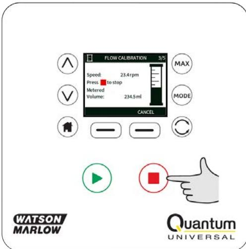
Use the  $\wedge$  /  $\vee$  keys to enter the actual volume of fluid pumped.
