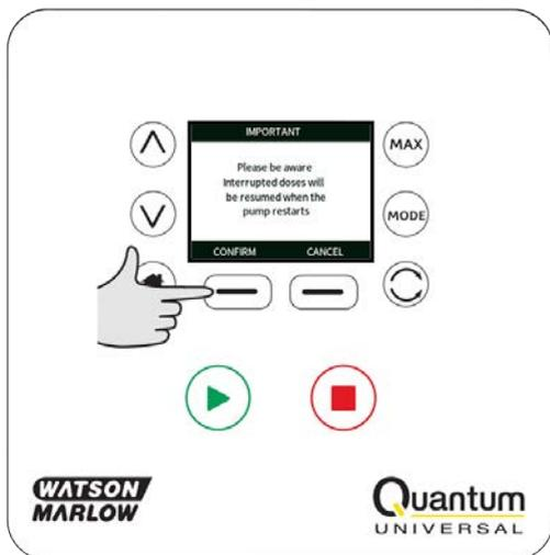
If resume interrupted doses has NOT been set the following warning screen is displayed, press **CONFIRM** to save this setting.
