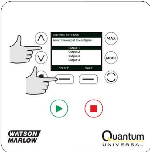
Use the  $\wedge$  /  $\vee$  keys and press **SELECT** to choose which pump status you require for the chosen output. The tick symbol indicates the current setting.
