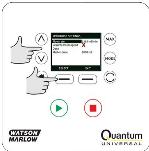
Using the  $\wedge$  /  $\vee$  keys, enter the dose flow rate and press **SELECT**.
