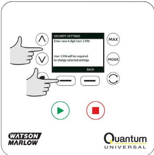
To define the allowed functionality, use the  $\wedge$  /  $\vee$  keys to select the functionality and press **ENABLE**. User 2 PIN will allow access to only the enabled functionality, to disable functionality, highlight the enabled functionality and press **DISABLE**. When all the required functionality has been enabled, press **FINISH**.
