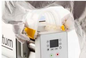
Lift the cartridge out of the pumphead.
