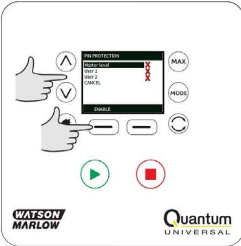
To define a four digit Master PIN, use the  $\wedge$ / $\vee$  keys to select each digit from 0-9. Once you have the required digit press the **NEXT DIGIT** key. After selecting the fourth digit press **ENTER**.
