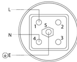
For installations that do not use the supplied mains lead, connect power using a suitably rated Harting PushPull Power® mating connection. To mate with Harting part 0935 231 0312 (internal connector). Cables should be current rated with respect to applied voltage, 100 to 120Vac : 10Amps, 200 to 240VAC : 6 Amps. Suggested cable size: 100-120VAC 1.3mm<sup>2</sup>, 220-240VAC 1.00mm<sup>2</sup>, 300V (minimum), 60C (minimum), VW-1 rated.
