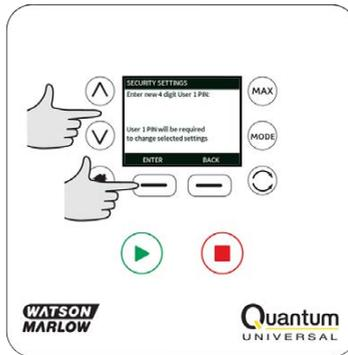
Now press **CONFIRM** to check that the number entered is the PIN you require. Press **CHANGE** to return to PIN entry.
