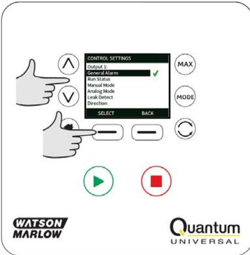
Use the  $\wedge$  /  $\vee$  keys and press **SELECT** to choose the logic state of the chosen output. Press **SELECT** to program the output or **BACK** to cancel.
