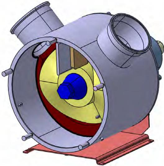
Loosen and remove the Shaft Nut
