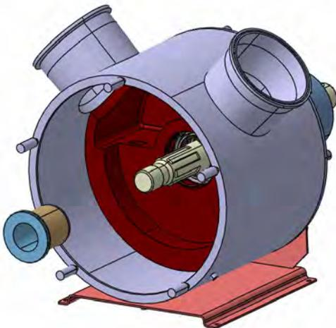
Remove the Shaft Sleeve
