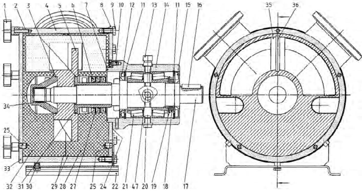
**26.6 Cross section drawing EC 60 with Mechanical Seal System**
