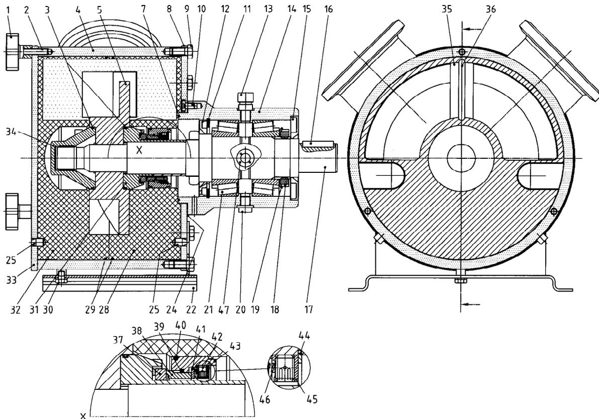
**26.5 Cross section drawing EC 60 with Lip Seal System**
