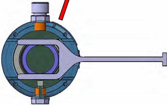
Before the work starts, the shaft has to be fixed against movement
