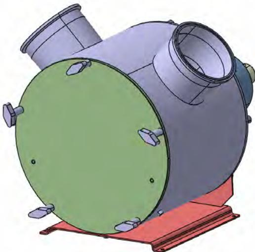
Remove Cap Nuts / Wing Nuts (RIGHT-HAND thread)
