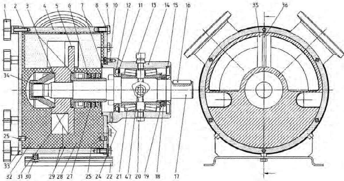
**26.4 Cross section drawing EC 40 with Mechanical Seal System**
