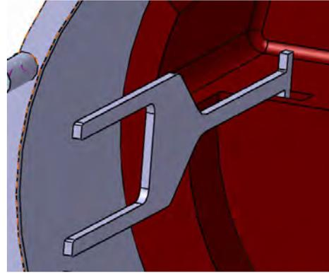
The nose of the tool has to be hooked in the groove of the Liner
