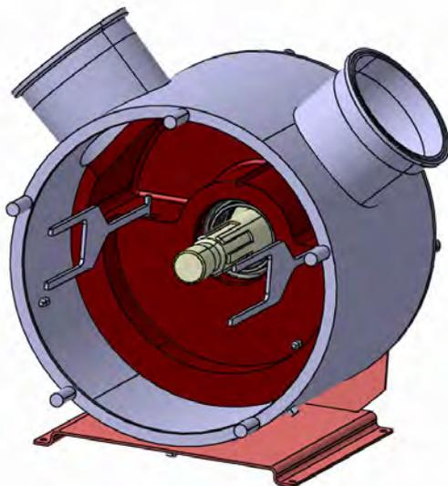
Remove the Liner, back with aid of tool kit
