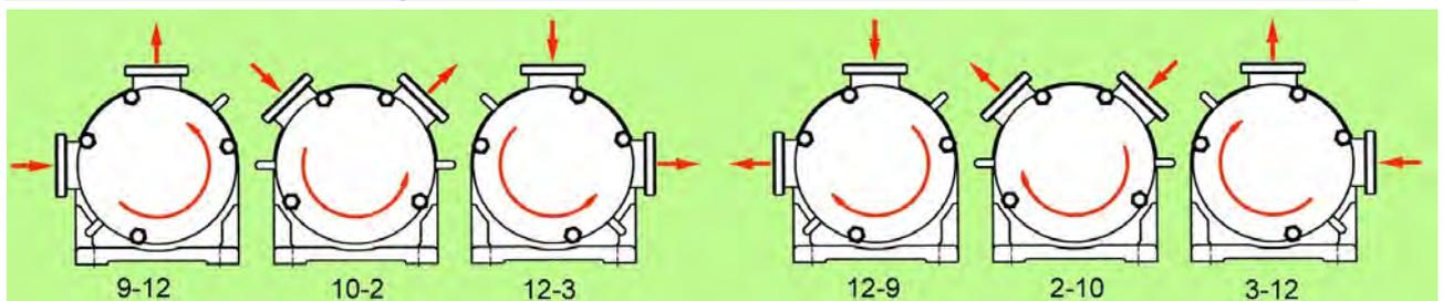
Counterclockwise rotation of the rotor and motor
