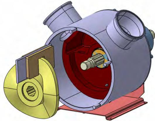
Remove the Rotor-Assembly, consisting of Rotor, Scraper and Guide Rail
