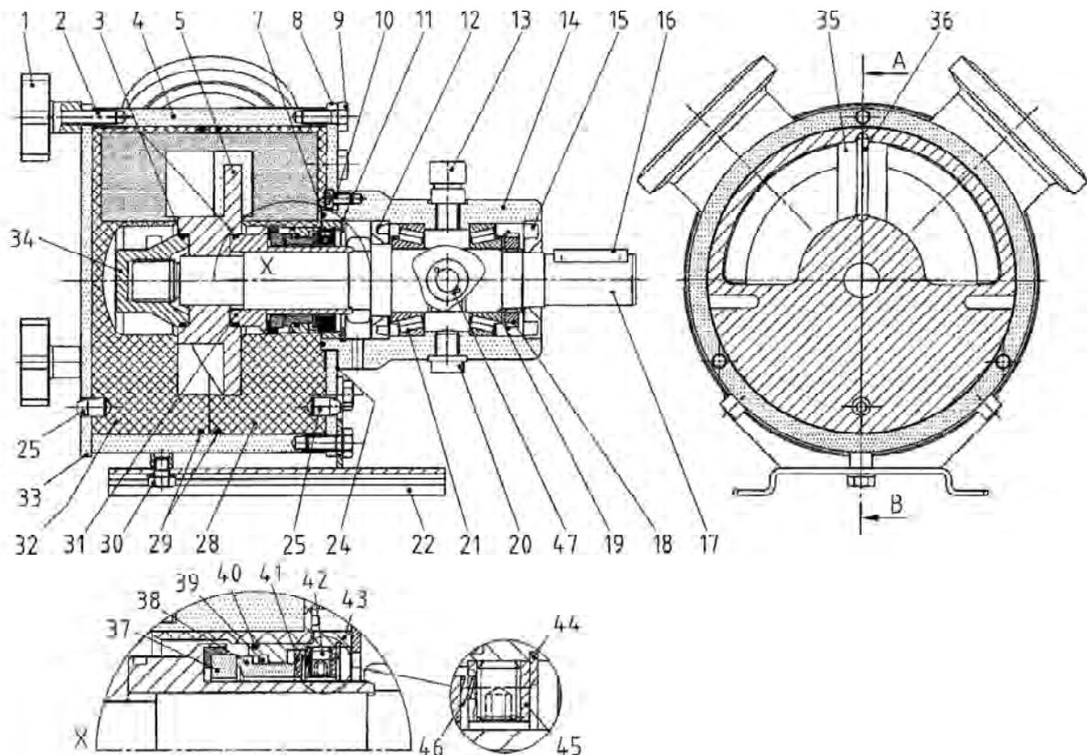
**26.3 Cross section drawing EC 40 with Lip Seal System**
