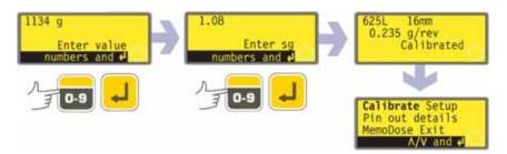
**Note**: If the pump has been set to display flow rate in units of mass (see 18.4 *Flow units*), as in this example, the pump displays a screen allowing you to confirm the specific gravity of the duty fluid immediately before the final press on **ENTER**.
