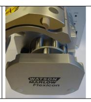
Open the dispenser head by tipping each of the two locking pins up and lift the tube bridge
