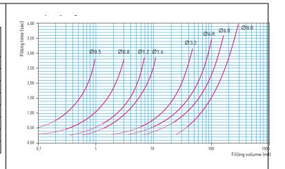
The filling time for a volume of 10.0 ml with a Ø3.2 ID tube is 0.8 seconds with dispenser running in high speed i.e. 400 in rpm and 100 in acceleration.
