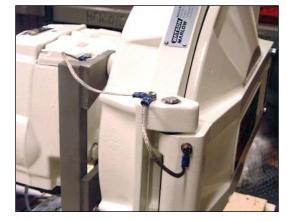
Electrostatic testing has shown that when this pump is used in conjuntion with Watson-Marlow Bioprene tubing, with dimensions for use in this pump, it is compliant with a II 2G c IIB T4 X rating. The X denotes that special instructions must be followed.
