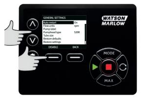
Use the  $\wedge$  /v keys to move the selection bar over **Pumphead** and press **SELECT**.
