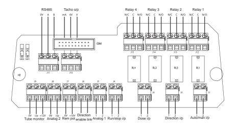
Recommended control cable: metric = 0.14 sq mm - 2.5 sq mm solid and 0.14 sq mm - 1.5 sq mm stranded. USA = 26AWG - 14AWG solid and 26AWG - 16AWG stranded. Cable: circular. Max/min outside diameter to ensure a seal when passed through the standard gland: 9.5 mm-5 mm. **The cable section must be circular to ensure a seal**.
