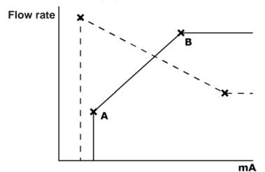
When the analog signal received is greater than the level defined by point A, the run status output will be energised as the pump is running.
