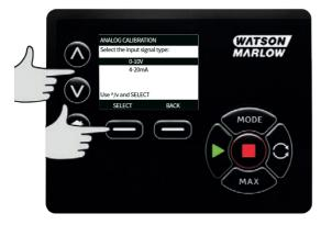
The pump gives the option to enter the high and low mA or V signals manually or via the analog input. Entering mA values is described here, however the process for entering V signals is identical. Choose whether to enter the current values manually via the keypad, or whether to apply the current signals electrically to the analog input.
