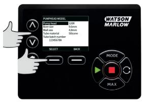
Use the  $\wedge$  / $\!\!\!\!\!\!\!\!\!\!\!\!\!\!\!\!\!\!\!\!\!\!\!\!\!\!\!\!\!\!\!$  keys to move the selection bar over the tube size to be used and press SELECT.
