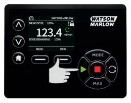
If the delivered dose differs from the volume required, the percentage may be adjusted within the limits 50% to 150% of the master dose. Use the  $\wedge l_{\gamma}$  keys to alter the percentage. The new dose size is displayed as a percentage on the home screen.
