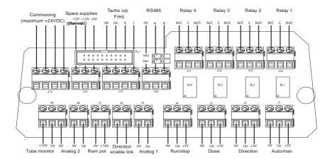
Note: It is recommended to separate the module from the pump and leave the connector PCB attached to the pump rear. Disconnect the Module ribbon from the pump by use of the ribbon eject levers on the connector board.
