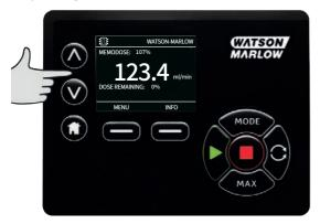
If **STOP** is pressed during dosing, the pump stops. Pressing **START** will resume, or discard, the interrupted dose depending on the settings in "Resume interrupted doses" on page 74.
