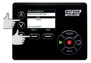
The pump gives the option to enter the high and low mA or V signals manually or via the analog input. Entering mA values is described here and the process for entering Voltage signals is identical. Choose whether to enter the current values manually via the keypad, or whether to apply the current signals electrically to the analog input.
