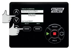
Using the  $\land$  /  $\lor$  keys, scroll to **Scaling input** and press **SELECT**.
