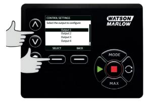
Use the  $\wedge$  / $\vee$  keys and press SELECT to choose which pump status you require for the chosen output. The tick symbol indicates the current setting.
