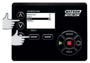
ENABLE user 2 security settings displays the PIN entry screen for User 2. To define a four digit User 2 PIN, use the  $\land$  / $\lor$  keys to select each digit from 0-9. Once you have the required digit press the **NEXT DIGIT** key. After selecting the fourth digit press **ENTER**.
