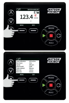
This will display the main menu as shown below. Use the  $\wedge$  / $\sim$  keys to move the selection bar between the available options.
