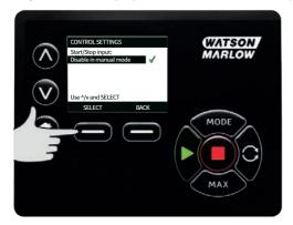
Use the  $\wedge$  /v keys and press SELECT to choose the logic state of the chosen input for your connected control hardware.
