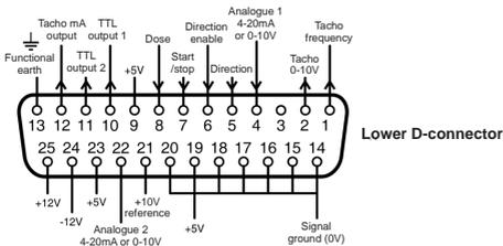
The 0V of this pump is DC isolated (floating) from the pump mains Earth. However, do not allow pump 0V to exceed 10V from the pump mains earth through connection with remote equipment, to avoid overstressing internal 0V to Earth EMI capacitors.
