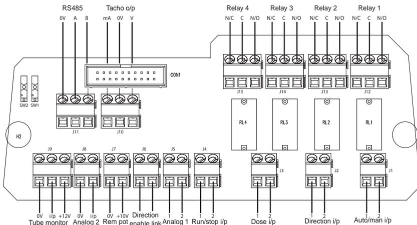
Recommended control cable: metric = 0.14sq mm - 2.5sq mm solid and 0.14sq mm - 1.5sq mm stranded. USA = 26AWG - 14AWG solid and 26AWG - 16AWG stranded. Cable: circular. Max/min outside diameter to ensure a seal when passed through the standard gland: 9.5mm-5mm. **The cable section must be circular to ensure a seal.**
