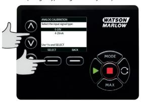
The pump gives the option to enter the high and low mA or V signals manually or via the analog input. Entering mA values is described here, however the process for entering V signals is identical.
