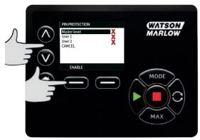
ENABLE user 1 security settings displays the PIN entry screen for User 1. To define a four digit User 1 PIN, use the  $\land / \lor$  keys to select each digit from 0-9. Once you have the required digit press the **NEXT DIGIT** key. After selecting the fourth digit press **ENTER**.
