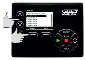
If a LoadSure element has been selected then the tube size is displayed as pressure and bore.
