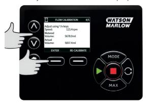
To accept the new calibration press **ACCEPT** or **RE-CALIBRATE** to repeat the procedure. Press **HOME** or **MODE** to abort.
