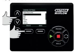
If a mass flow unit is selected, the specific gravity of the fluid must be entered. The following screen is displayed.
