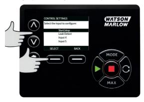
The default is  $\star$ . The start/stop input is not disabled in manual mode. Press **SELECT** to change the setting to  $\checkmark$ .
