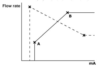
When the analog signal received is greater than the level defined by point A, the run status output will be energised as the pump is running.
