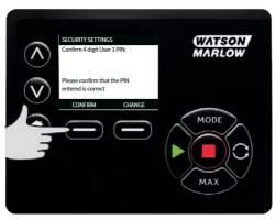
To define the allowed functionality, use the  $\land \land \lor$  keys to select the functionality and press **ENABLE**. User 1 PIN will allow access to only the enabled functionality, to disable functionality, highlight the enabled functionality and press **PISABLE**. When all the required functionality has been enabled, press **FINISH**.
