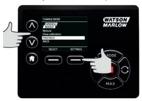
Use the  $\land$  and  $\lor$  keys to alter the station address, in the range from 1 to 125 (126 is the default station address). Press **FINISH** to set the station address, or **NEXT** to enable/disable PROFIBUS communication.
