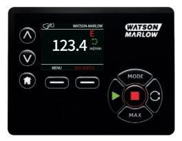
The MODE button gives access to the PROFIBUS settings and the station address. When the menus are accessed, the pump is technically still in MANUAL mode but with no PROFIBUS communications. After five minutes of inactivity the pump will revert back to the MANUAL home screen and discard any unsaved changes, if there are still no communications then the red P icon will be displayed. For further information on PROFIBUS communication errors see section "PROFIBUS communication errors" on page 47.
