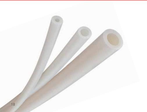
PTFE-reinforced fluoroelastomer tubing which handles nearly all aggressive chemicals, including organic solvents such as methyl ethyl ketone, toluene and acetone. With 50 times longer life than other fluoroelastomers and pressures up to 4 bar.
