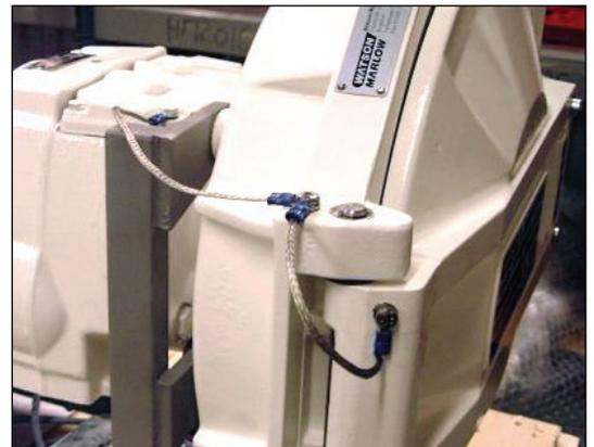
Electrostatic testing has shown that when this pump is used in conjunction with Watson-Marlow Bioprene tubing, with dimensions for use in this pump, it is compliant with a II 2G c IIB T4 X rating. The X denotes that special instructions must be followed.
