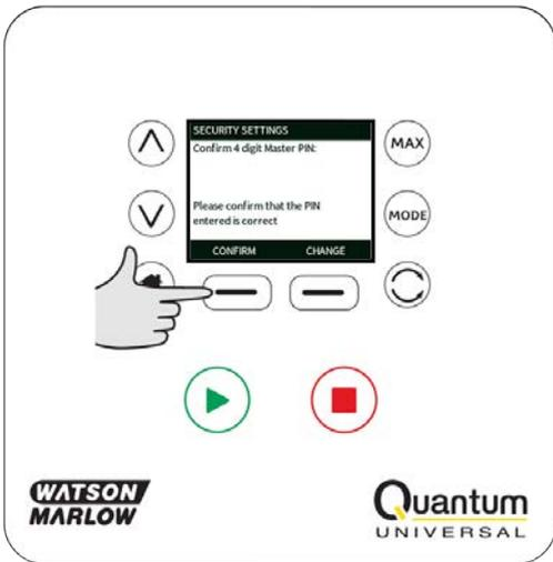
The following screen will be displayed to indicate that the Master PIN has been applied to access all functionality. Press **NEXT** to selectively enable functionality access for User 1 and User 2.
