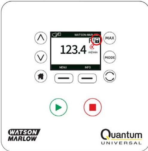
Note that the STOP key will always work whether the keypad is locked or not.
