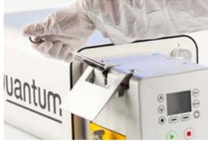
Using the spanner supplied, release the Quantum Track Handles on the pumphead.
