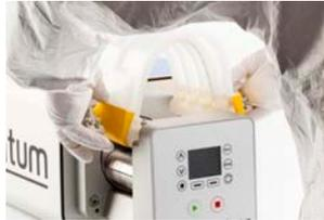
Lift the cartridge out of the pumphead.
