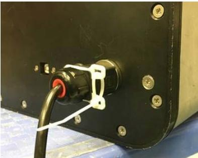
Ensure the security clip is secured to the power connector with a tie wrap (as shown) and the Harting power connector is in place before power is applied to the unit.
