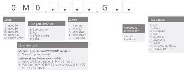
\* The pumphead side location is required when ordering. The left/right perspective assumes the user is looking at the front of the pump. The pump in the dimensions diagram is considered a pumphead located to the left.
