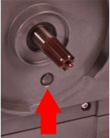
Check the leak detect sensor and driveshaft are clean and free from process chemical. If any evidence of chemical residue is found, remove the pump from service and contact your local Watson-Marlow representative for advice.
