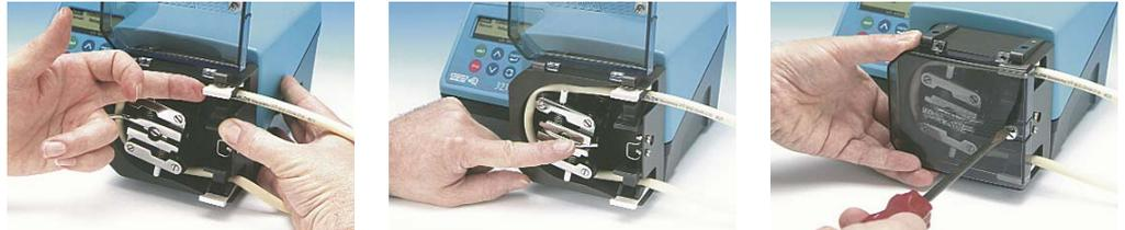
The tube clamps can accommodate various tube diameters by pushing in, or pulling out, the grip bars within the clamp. Set the clamps to apply the minimum necessary pressure to the tubing.
