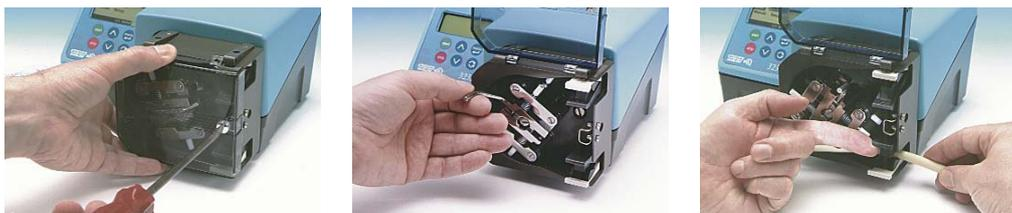
The rotor has tube guide rollers that pull the tube into the pumphead during loading. Turn the rotor carefully until the tube guides pick up the tube. Continue to turn the rotor, and feed the tubing in between the guides.
