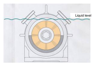
The pump must always be filled with the corresponding medium before commissioning and during operation, with the liquid level above the rotor (see diagram). The filling of the pump should be done outside the combustible area.
