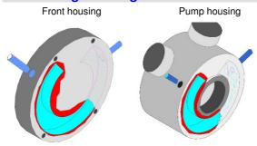
There is a crescent-shaped channel milled into the housing which is sealed later by a stainless steel plate. There are connections on two sides through which the heating or cooling agent flows. Counterpressure should not exceed 1 bar. You can dictate temperature and pumping rate by the heating or cooling agent.
