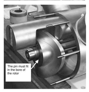
Push the rotor, the gate and the gate guide as one unit into the housing. Make sure that the gate guide and the gate are in the correct installation position. (Refer to the ROTATION DIRECTION CHANGE chapter)
