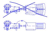
Place the pump on a <u>level</u> ground.
