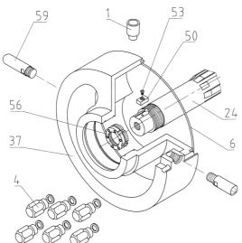
The innards of the pump are now in front of you. I.e., you can see the gate guide, the gate, the shaft sleeves, the rotor and the two halves of the liner.
