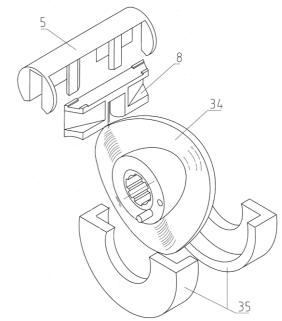
The remaining parts and the second half of the liner can also be axially pulled from the shaft or the pump housing.
