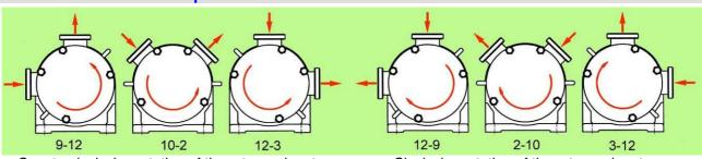
Counterclockwise rotation of the rotor and motor
