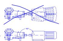
Align the shaft of the pump with the shaft of the drive.
