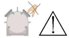
Rotating rotor in the pump. Danger of crushing or cutting off fingers and hands. The pump must be protected by the customer so that it is not possible for persons to grasp in the opening with the rotor running. In the case of work on the stationary Rotor, the drive must be secured against unintentional switching on. Increased danger exists with dismantled pipes and opened pump.
