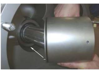
The pin has to be fixed in the groove in the pump housing
