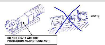
Place the pump on a level ground.
