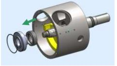
The dynamic unit of the mechanical seal can be removed. Be careful with the faces.
