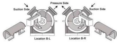
If the Rotor turns counter clockwise
