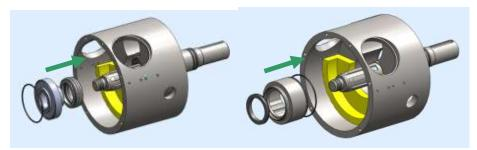
Fit the seal face in the stainless steel static part. Fit the bellow into the stainless steel dynamic part.
