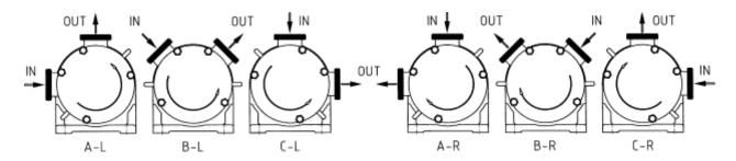
Counterclockwise rotation of the rotor and motor Clockwise rotation of the rotor and motor Unless otherwise ordered, the pump is delivered in position B
