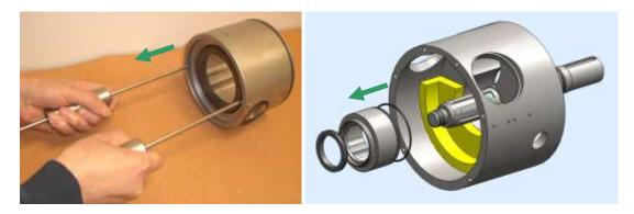
Now the complete seal system can be pulled out of the back of the pump housing for replacement or inspection. Use removal tool S60-9003-12.
