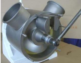
tighten the locking nut with the torque of 160 Nm
