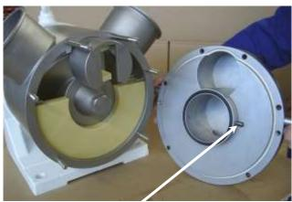
The pin of the front bearing has to be fixed of the groove in the front cover
