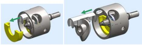
After opening the front cover and the locking nut as described in the manual, pull the front liner out of the pump housing, remove the rotor together with the scraper gate and scraper gate guide.
