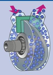
A single sinusoidal rotor creates four evenly sized chambers as it rotates. Fluid is "pulled" through the inlet into each chamber in turn. As the chamber rotates, it contracts, closes then discharges fluid through the outlet port. At the same time, the opposite chamber opens to draw in more fluid, resulting in a smooth flow with virtually no pulsation.
