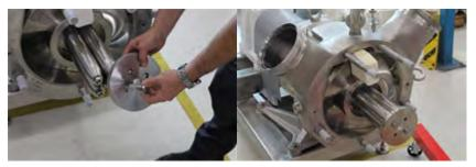
• The fixation plate can be used as a stopper
