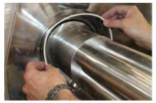
• Fit the O-ring to the inner diameter of the back housing.
