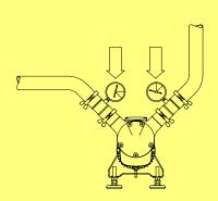
MasoSine pumps normally run with such a low resonant frequency that no damage results. However, particularly when running with inverters, certain frequencies can cause interference vibrations which must be avoided. It is important during commissioning to ascertain whether such vibrations exist and to define them, so that the inverter can be programmed to avoid these frequencies. Similarly, interference from cavitation or rigid lines must be avoided.
