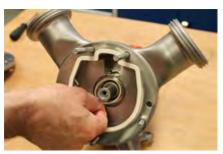
• Insert the O-ring into the groove of the O-ring holder.
