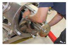
• Pull the rotor, together with the gate, out of the housing, as shown.
