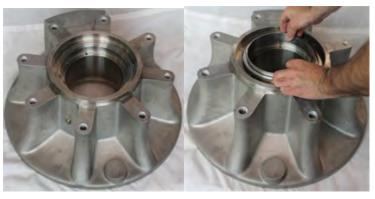
The flush ring in the back of the flange. This is used with the single mechanical seal system. A lip seal is placed in the ring in the same way as a flush ring for a flush system.
