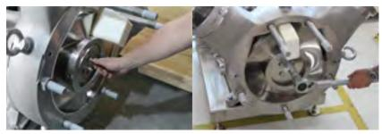
Insert the fixation plate and fasten the screws.
