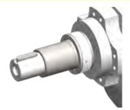
The pin correctly fitted into the notch.
