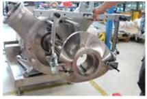
Carefully remove the rotor and store safely. Take care when removing the rotor to ensure the seal faces are not damaged.
