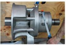
• Tighten the screws on the support at the back of the housing, by turning them clockwise with a wrench.
