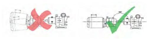
• Align the pump shaft with the drive shaft.
