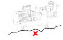
• Place the pump on a level surface
