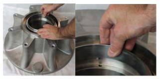
The spring assembly correctly assembled in the rear of the back housing.
