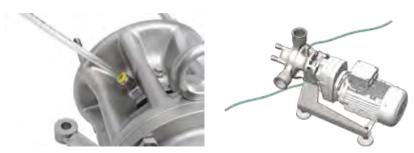
The picture shows a tube connected for the flush system. The tubing should have an outer diameter of 8mm or connection with G1/8 thread.
