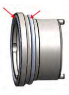
O-ring receptacle with 2x O-ring in the groove on the face and on the outer diameter. This is inserted into the pump housing. Note: EPDM components cannot withstand oil and grease.
