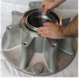
• Install the spring assembly in the rear of the back housing. Make sure that the pins fit into the notches.
