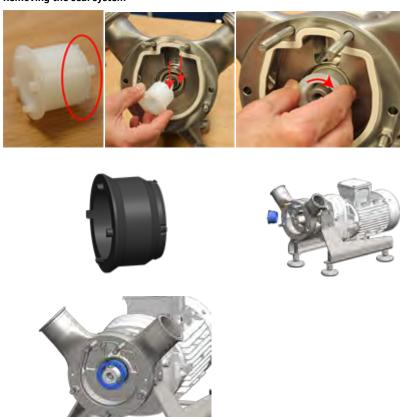
• Insert the tool (TL-Cxxx-001-50) with the claws into the grooves and turn clockwise by 45°.
