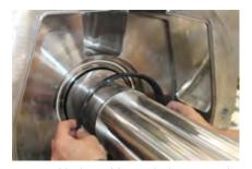
$\bullet \quad \text{Assemble the seal face in the housing. Make sure the small pin fits into the notch on the seal face.}\\$
