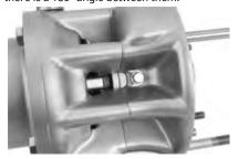
Plug all other possible connections on the frame, using the threaded plugs supplied with the pump (see "Parts lists" on page 54 for the part numbers). The other connections are intended for use with different orientations of the pump's nozzles (see "Possible pump orientations" on page 19).
