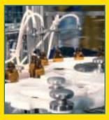
Reliability and easy cleaning are important features of Watson-Marlow Bredel peristaltic pumping, according to Dales Pharmaceuticals, who use a 500 series dispensing pump to package a wide range of pharmaceutical preparations. Before taking delivery of their new pump, Dales used a pneumatic machine to dispense volumes varying from 10ml to 100ml, of 10 major fluids.
