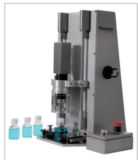
FCE50L with an illuminating start button to show that required torque has been acheived
