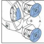
Place a tray (A) under the drain plug in the cover of the pump. Remove the drain plug (B). Catch the lubricant from the pump housing in the tray. Position the drain plug and tighten it firmly.
