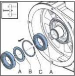
9. Remove the seal (A). Clean and degrease the bore.
