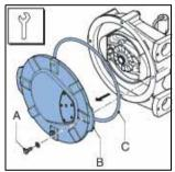
5. Loosen the retaining bolt (A) of both pressing shoes (B). Remove the shims (C) if present.
