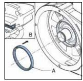
11. Check that the hub is clean and free of grease. Fit the bearings and the rings now.
