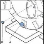
3. The pump housing can be filled with lubricant via the breather/vent (A) on the rear of the pump housing. For this purpose remove the breather cap (B) and position a funnel (C) in the breather. Pour the lubricant in the pump housing via the funnel.
