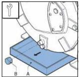
4. Remove the cover (B) by loosening the retaining bolts (A).
