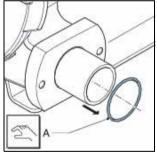
10. Power out the hose (A) from the pump chamber by jogging the drive motor.
