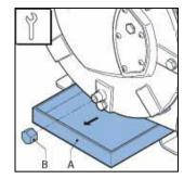
Position the drain plug (A) and tighten it firmly.
