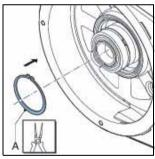
13. Fit rotor (A). The rotor is placed on the bearings with a loose fit. Press the rotor on the hub until it sticks.
