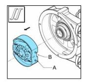
7. Dismount the retaining circlip (A) with the correct tool.
