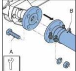
5. Loosen hose clamp (A) of both the inlet and outlet ports by loosening retaining bolt (B).
