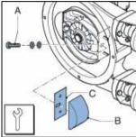
Fit the removed shims (C) again. Position the (new) pressing shoe (B), check that the Nord-Lock<sup>®</sup> rings (D) have been positioned correctly and tighten the retaining bolt(s) (A) a few turns. Refer to § 10.1.7.
