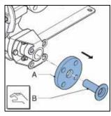
Loosen the retaining bolts (A) of the flange bracket (B) and remove the bolts. Slide the flange bracket and the hose clip (C) off the hose. Carry out this procedure both for the inlet and outlet ports.
