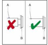
Now fully tighten the retaining bolts (A) of the flange bracket (B). Make sure the bolts are tightened with the correct torque. Refer to § 10.1.7.
