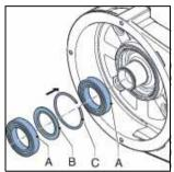
12. Mount the retaining circlip (A).
