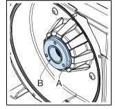
7. Fit the (new) rotor (B) on the pump shaft (C). Install the retaining bolts and washers (A) and tighten them to the correct torque. Refer to § 11.1.6.
