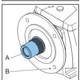
Use circlip pliers to remove the circlip (A) from the pump shaft (B) and, if the bearing must be replaced, to remove the circlip (C) from the pump housing (D).
