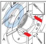
9. At the front of the pump housing, place a suitable bush (A) against the outer ring (B) of the bearing. The outer diameter of the bush (A) must be 103 ±1 mm. Use a plastic hammer to gently drive out the bearing.
