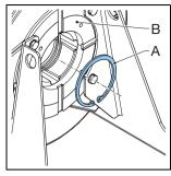
13. Slightly grease the sealing lip of the (new) dynamic seal (A). Do not grease the outside surface of the dynamic seal. Fit the dynamic seal from the front side in the pump housing, using good engineering practices. The seal ring must be fitted in the correct orientation. Make sure that the open side points towards the pump cover.
