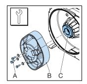
Check the outside of the dynamic seal (A) for deformation or damage as far as possible. The dynamic seal is partly covered by the pump shaft. Replace the dynamic seal if necessary. Refer to § 8.6.2.
