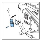
Mount the breather (A) with high-level float switch.
