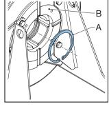
Slightly lubricate the contact surface of the inner 14. ring of the bearing (A) and the pump shaft (B). Position the pump shaft in the bearing. Gently tap on the pump shaft until the collar touches the bearing. Use a plastic hammer.
