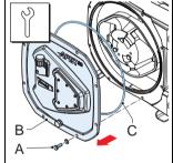
4. Remove the nut (A) and the old sensor (B).
