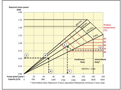
A: Required flow or pump speed
