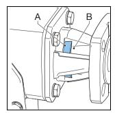
Lubricate the insert (A) with Bredel Genuine Hose Lubricant. Manually spread the lubricant over the insert.
