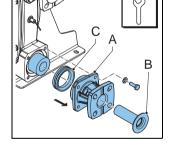
9. Drive out the hose (A) from the pump housing by jogging the drive motor.
