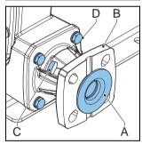
11. Tighten the bolts (A). Normally, it is sufficient to tighten two bolts that are diagonally opposite each other. The other two bolts can be tightened when the bracket is at its end position. Make sure the bolts are tightened to the correct torque. Refer to § 11.1.6.
