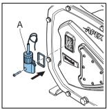
3. Connect the high-level float switch to the auxiliary power circuit via the 1.5 metre long PVC cable (2 x 0.34 mm²). Bear in mind that the electrical contact of the float switch is normally closed (NC). The knob is upwards for normally closed operation. When the lubricant level is (too) high the contact will open.
