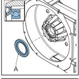
15. Install the (new) O-ring (A) in the pump shaft.
