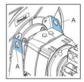
The complete hose pump, i.e. pumphead, gearbox and electric motor, must be lifted using the lifting eyes and suitably rated straps or slings (A). For the weights, refer to § 11.1.5.
