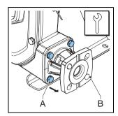
Pull the insert out of the hose. If necessary, insert the tip of a screwdriver behind the flange of the insert.
