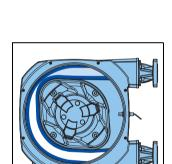
In phase 3, the second integral pressing shoe compresses the pump hose. Due to the continuous rotating movement of the rotor new fluid is sucked in and fluid that is previously drawn in is pressed out by the shoe. When the first shoe leaves the pump hose, the second shoe has already occluded the pump hose and fluid is prevented from flowing back. This method of liquid displacement is known as the "positive displacement principle".
