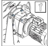
Check the teeth on the coupling bush (A) that is on the output shaft of the gearbox (B) for wear and damage. Replace the coupling bush if necessary.
