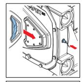
3. Remove the cover (B) and the O-ring (C) by loosening the retaining bolts (A).
