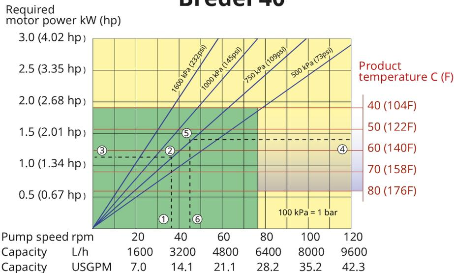
Note: The area of continuous operation diminishes with increased product temperatures. For product temperatures >40C, the area of continuous operation reduces to the corresponding red temperature line.
