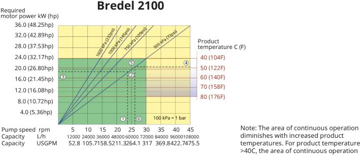
diminishes with increased product temperatures. For product temperatures >40C, the area of continuous operation reduces to the corresponding red temperature line.
