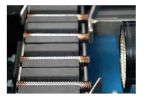
In addition, Aflex has developed a fully automated inspection system which verifies the internal bores, braid outer diameter, flare diameter and hose length, ensuring only products that are 100% fit for purpose are sent to the customer. This inspection system is only applicable to regularly supplied large quantities of cut lengths and is limited to cut length which are less then 150mm (5.9 inches) in length.
