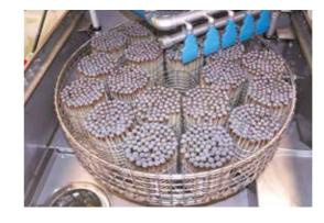
Automated washing equipment is available for the cut lengths, which has the capability of achieving the required tolerance levels, whilst our validation equipment allows Aflex to verify the particle size, particle count and particle weight. Tolerance levels are typically 85 particles between 150 and 400 microns – with our facilities we typically find 0-5 particles of this size upon inspection.
