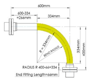
Note: The bend radius is measured to the inside edge of the hose, For the minimum bend radius refer to page 6.
