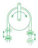
The Fourth Rule is that the hose must not be subjected to torque, either during connection, or as a result of the flexing cycle.
