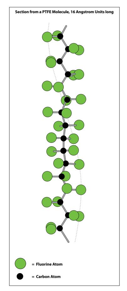
PTFE, or Polytetrafluoroethylene, comprises of longchain molecules of carbon atoms, each linked to two fluorine atoms.
