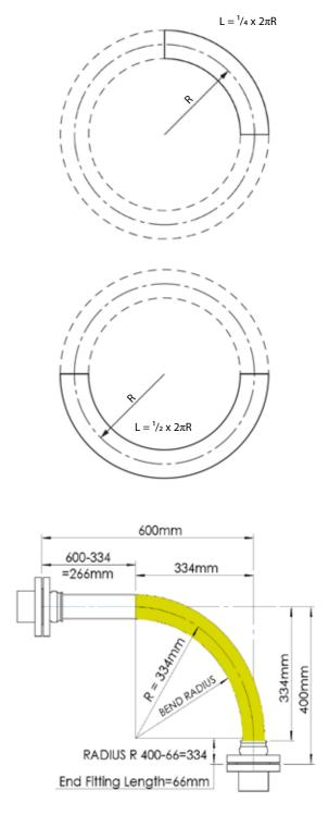
Note: The bend radius is measured to the inside edge of the hose, For the minimum bend radius please refer to page 8.
