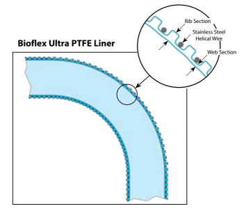
Note - The new designs with the increased bores and the helical wire reinforcement only apply to the standard products. The 3/8" size will remain the same as before, with nominal bore size and no helical wire reinforcement.
