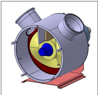
Loosen and remove the Shaft Nut
