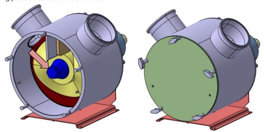
The pump needs to be completely assembled. The shaft nut (red arrow) needs to be mounted with the required torque.
