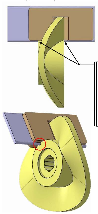
During mounting of the Rotor-Assembly the noses of the Guide rail mustn't be laid on the surface of the Rotor. To achieve this you have to fit Scraper and Guide rail in a position that the noses of the Guide rail are touching the gable end of the Rotor.
