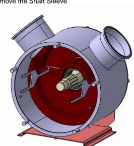
Remove the Liner, back with the aid of tool kit
