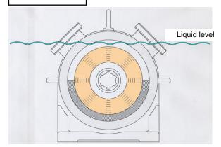
The pump must always be filled with the corresponding medium before commissioning and during operation, with the liquid level above the rotor (see diagram).
