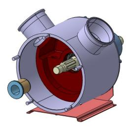
Remove the Shaft Sleeve
