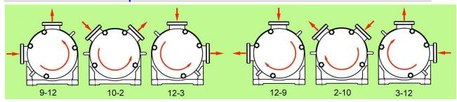
Counterclockwise rotation of the rotor and motor
