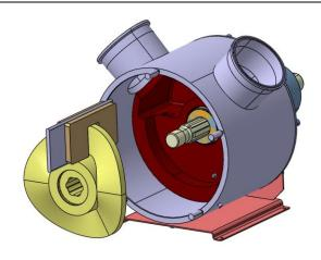
Remove the Rotor-Assembly, consisting of Rotor, Scraper and Guide Rail
