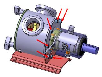
If the pump is completely disassembled and the flange is detached from the housing, the following steps must be done to ensure centering the liners to the shaft. Otherwise this may lead to a leakage of the sealing system.
