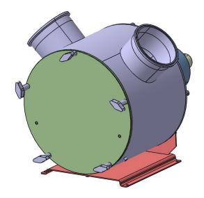
Remove Cap Nuts / Wing Nuts (RIGHT-HAND thread)
