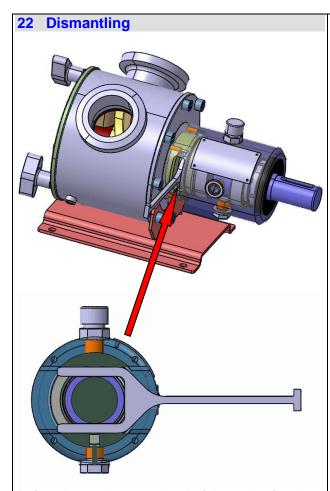
Before the work starts, the shaft has to be fixed against movement
