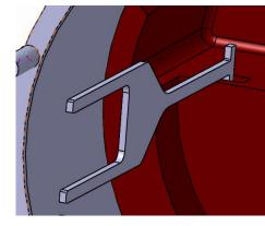
The nose of the tool has to be hooked in the groove of the Liner
