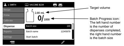
If Start batch is highlighted press to start the batch. If reporting is **On**, a batch report will be created.
