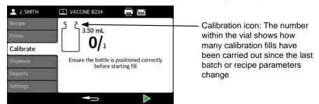
The pump uses the current recipe parameters during the calibration process, i.e. volume, density, tube size, speed, acceleration, deceleration, and anti-drip. The units used in calibration can be volume or mass and are set through the settings tab.
