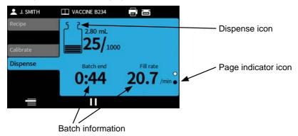
Use the up and down keys ( $\wedge/\vee$ ) to change the information that is displayed whilst a batch is running.
