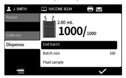
If **End batch** is highlighted press to end the batch. If reporting is **On**, the batch report will be completed.
