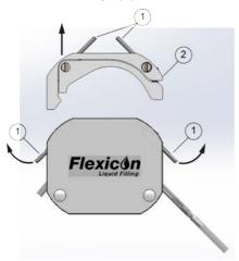
2. Mount the correct tube lock (3) on its dowel pin and place the correct tubes in the dispenser head.
