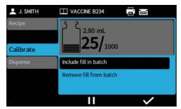
If the bottle used for calibration should be included in the batch, highlight **Include** in batch and press
