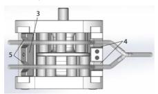
3. Looking towards the pump head from the front. The Y-connector must be situated to the right of the dispenser head.
