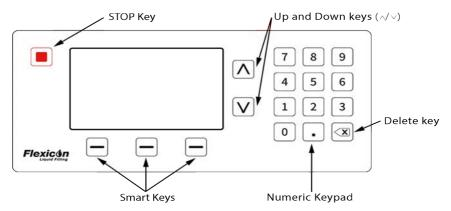
The **STOP key** will immediately stop the pump, regardless of what screen is currently displayed. If the pump is stopped part way through a fill, a message stating this will be displayed.
