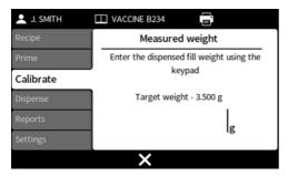
If not using a balance connected to the pump, enter the dispensed value using the numeric keypad and press
