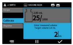
If not using a balance connected to the pump, enter the calibration value using the numeric keypad and press
