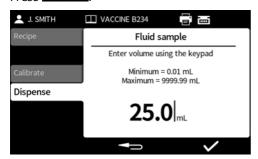
Enter the desired value and press . The fluid sample can then be dispensed.
