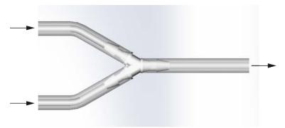
When the Y-connector has been assembled, mount the tubes in the dispenser head as shown below.
