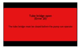
The tube bridge must be closed for the warning screen to clear and the pump to start.
