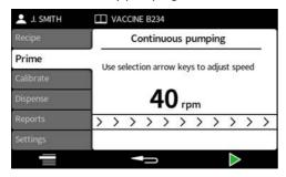
Adjust the pump speed using the up and down keys ( $\sqrt{\ }$ ).
