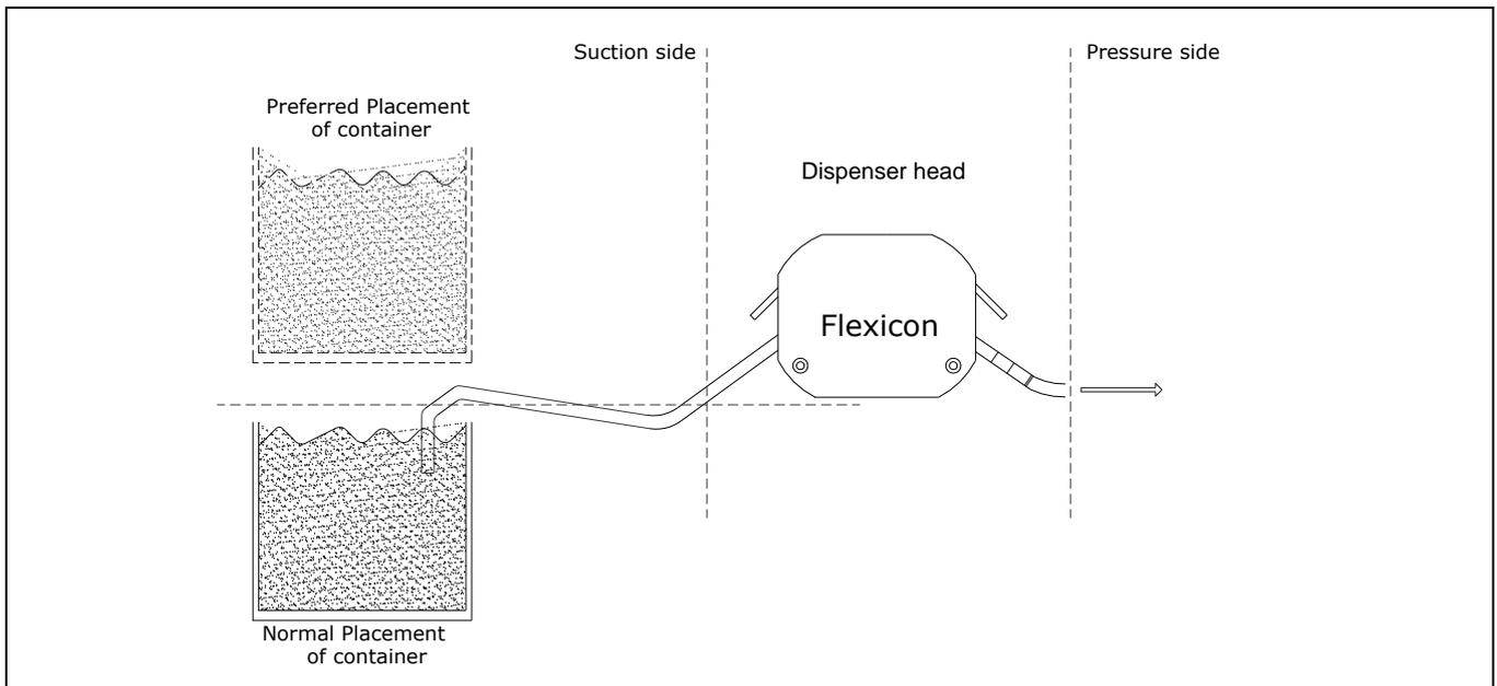
**Fig. 5 - placing the product container**
