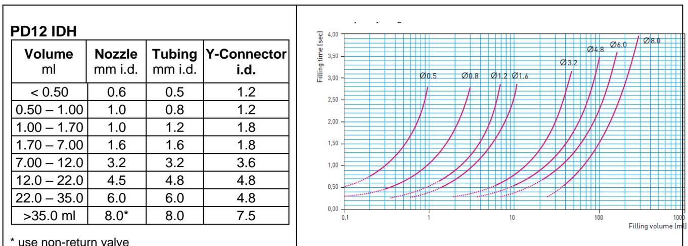
The filling time for a volume of 10.0 ml with a Ø3.2 ID tube is 0.8 seconds with dispenser running in high speed i.e. 400 in rpm and 100 in acceleration.
