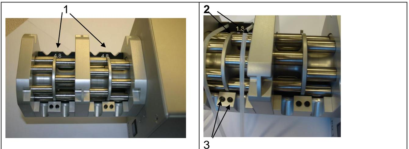
Mount the correct tube lock (1) on its dowel pin and place the tubes.
