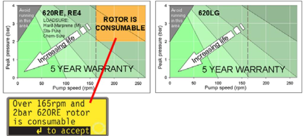
This pump's default running speed is 165rpm. It can be run at any speed up to 265rpm. Please note, however:
