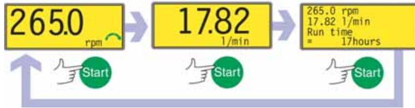
If the pump is running when **START** is pressed, it causes the information shown on the manual mode main screen to cycle from revolutions per minute, to flowrate in a choice of units (via a warning screen if flowrate has not been calibrated and if this is the first cycle since power-up) to rpm, flowrate and Run time. An example is shown here. The default can be altered from within the Setup menu (see 18.3 *Display*).
