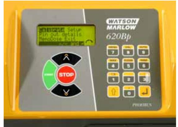
**Note:** Confirmation screens are displayed for 4 seconds. While they are displayed, a single press on any key removes them.
