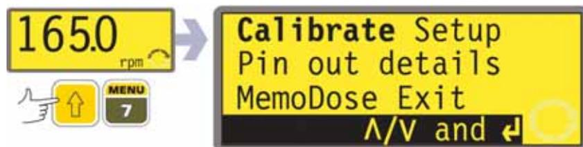
The main menu offers five options: **Calibrate**, **Setup**, **Pin out details**, **MemoDose** and **Exit**. Use the **UP** and **DOWN** keys to make a choice. Press the **ENTER** key to confirm your decision.
