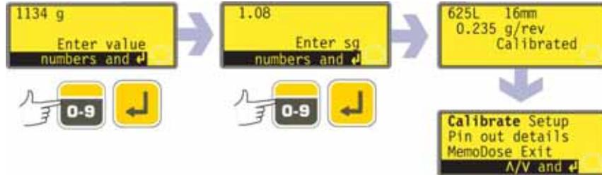
**Note:** If the pump has been set to display flow rate in units of mass (see 18.4 *Flow units*), as in this example, the pump displays a screen allowing you to confirm the specific gravity of the duty fluid immediately before the final press on **ENTER**.
