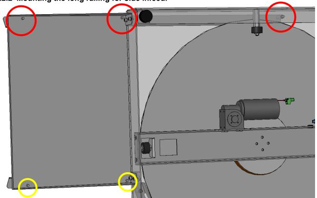
The FF20 comes with a short railing mounted on the infeed tray- yellow circles. There are 2 long railings: 1 for side infeed and 1 for front infeed.
