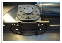
Loosen the 4 bolts underneath and move the motor to the left until the belt is tense again.\*
