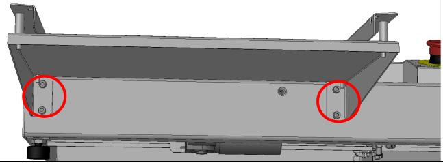
3.3.2.4 Mounting the long railing for side infeed.
