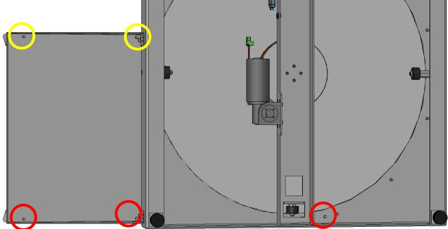
The FF20 comes with a short railing mounted on the infeed tray- yellow circles. There are 2 long railings: 1 for side infeed and 1 for front infeed.
