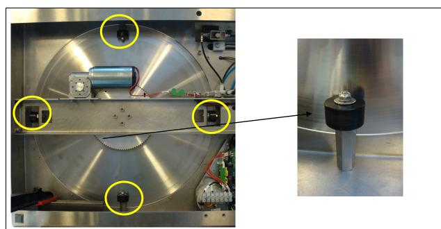
Turn of power, remove all connections to other equipment and tip the FF20 to gain access to the plastic rollers.
