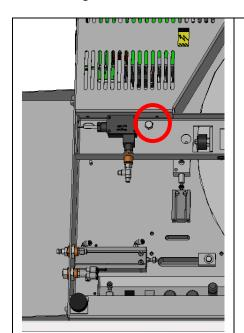
Fasten the bolt underneath the base plate.
