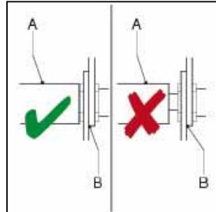
8. Tighten the bolt (A) of the hose clamp (B). Make sure the bolt is tightened with the correct torque. Refer to § 10.1.7.
