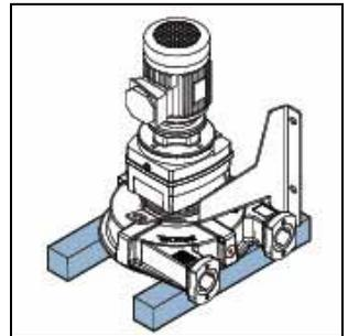
6. Remove the nuts (B), washers (C) and the pump drive (A).
