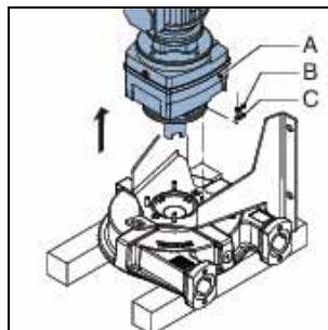
7. Put a plastic or wooden drive pin (A) on the rotor.
