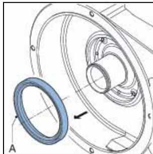
13. Fit a new seal ring (A) using good engineering practises. The seal ring must be fitted in the correct orientation (B). Make sure that the open side points to the pump cover.
