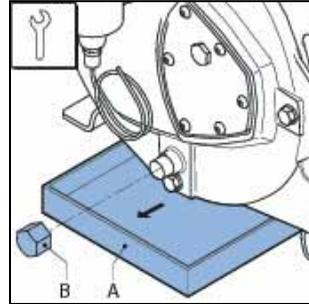
2. Position the drain plug (A) and tighten it firmly. For DuCoNite® 15 and DuCoNite® 20, remove the breather plug (B) before filling the lubricant. The DuCoNite® 10 can be filled without de-aerating.
