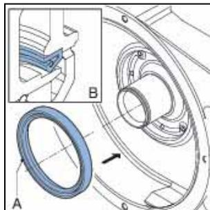
14. Check that the hub is clean and free of grease. Fit the bearings and the rings. The bearings are placed on the hub with a slight interference fit. Use a pressing tool to press the bearings on the hub.
