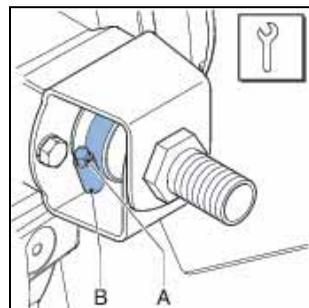
10. Fill the pump housing with Bredel Genuine Hose Lubricant. Refer to § 7.5.
