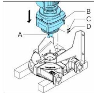
19. Fit the pump drive (B) with the nuts (C) and washers (D). Tighten to the specified torque settings. Refer to § 10.1.7.
