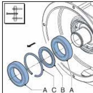
12. Remove the seal ring (A). Clean and degrease the bore.
