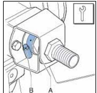
6. Loosen the retaining bolts (A) of the bracket (B) and remove the bolts.
