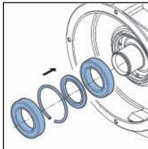
15. Mount the circlip (A).
