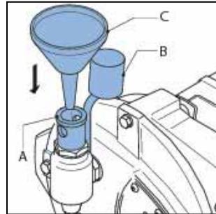
4. Keep on pouring until the lubricant level has risen above the level line in the inspection window.
