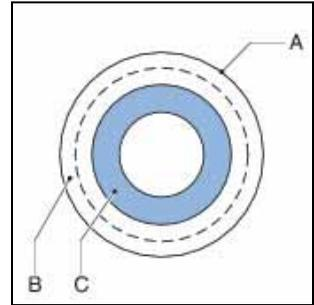
The pump hose liner material should be chemically resistant with the product to be pumped. Dependent on the specific requirements of your application a corresponding pump hose must be selected. For each pump model various hose types are available.
