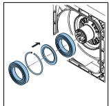
15. Mount the circlip (A).
