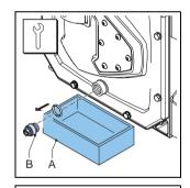
The pump housing can be filled with lubricant via the breather (A) on the cover. For this purpose remove the breather cap (B) and position a funnel (C) in the breather. Pour the lubricant into the pump housing through the funnel.
