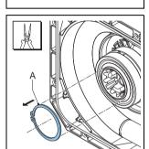
Dismount the bearings (A), the spacer ring (B) 11. and the retaining ring (C) with the correct tool. Clean the hub.
