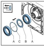
12. Remove the seal ring (A). Clean and degrease the bore. The holes in the pump housing can be used to drive out the old seal.
