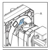
The complete hose pump, i.e. pumphead, gearbox and electric motor, must be lifted using the lifting eye plus additional support using suitably rated straps or slings (A). For the weights, refer to § 11.1.5.
