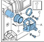
7. Turn the rotor in such a way that the hose (A) is pressed firmly against the bracket (B).
