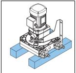
6. Remove the nuts (B), the washers (C) and the pump drive (A).
