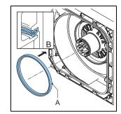
Slightly oil the inner ring of the (new) bearings and the seat on the hub. Fit the bearings and the rings.
