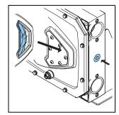
3. Remove the cover (B) by loosening the retaining bolts (A).
