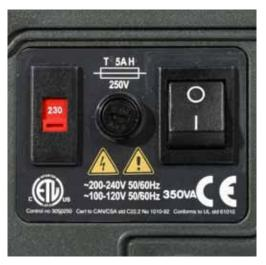
**Input line fusing**: type T5A H 250V 20mm time-delayed cartridge fuse, located in a fuseholder in the centre of the switchplate at the rear of the pump.
