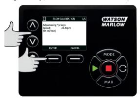
Press **START** to begin pumping a volume of fluid for calibration.
