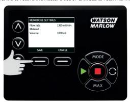
When MemoDose SETTINGS are complete the following screen is displayed; press **MEMODOSE** to start in MemoDose Mode or **BACK** to return to MemoDose settings.
