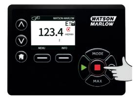
Stops the pump. The display background changes to white. If the pump is not running pressing this has no effect.
