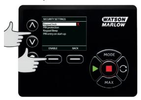
Once locked it will display the screen below when any key is pressed. To unlock the keypad press the two **UNLOCK** keys together.
