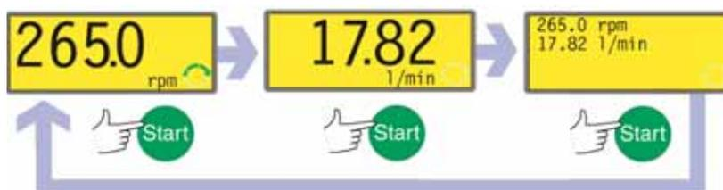
If the pump is running when **START** is pressed, it causes the information shown on the manual mode main screen to cycle from revolutions per minute, to flowrate in millilitres per minute (via a warning screen if flowrate has not been calibrated and if this is the first cycle since power-up) to rpm and flowrate. An example is shown here.
