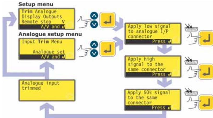
When the pump is under remote control, it tracks an analogue signal from the user's remote control system to the **i/p** terminal of the Analogue 1 connectors at the rear of the pump within the ranges 4-20mA, 0-10V or 1-5V. The **Trim** setup sequence allows the user to customise the process-signal-to-pump-speed calibration. The sequence may be entered directly from the Setup menu or from the Analogue setup menu.
