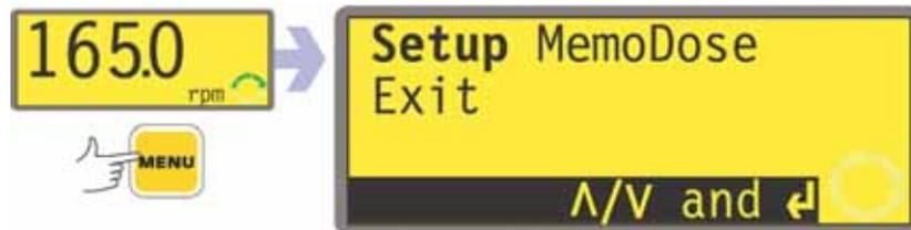
The main menu offers three options: **Setup**, **MemoDose** and **Exit**. Use the **UP** and **DOWN** keys to make a choice. Press the **ENTER** key to confirm your decision.
