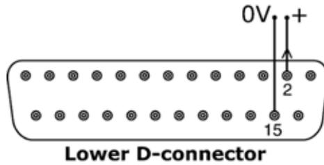
An analogue output signal is available as a 0V-10V signal on pin 2 of the lower D-connector. Ground to pin 15. The voltage is fixed and directly proportional to the pumphead rotation speed. 0V = zero speed; 10V = maximum speed.
