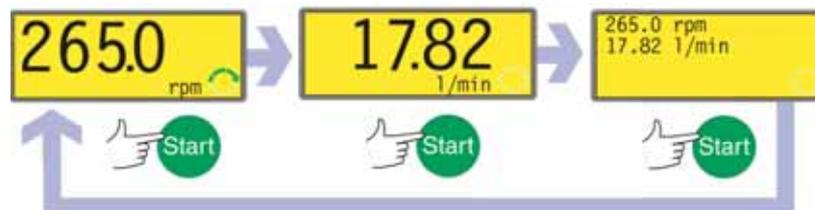
If the pump is running when **START** is pressed, it causes the information shown on the manual mode main screen to cycle from revolutions per minute, to flowrate in a choice of units (via a warning screen if flowrate has not been calibrated and if this is the first cycle since power-up) to rpm, flowrate and Run time. An example is shown here. The default can be altered from within the Setup menu (see 16.3 *Display*).
