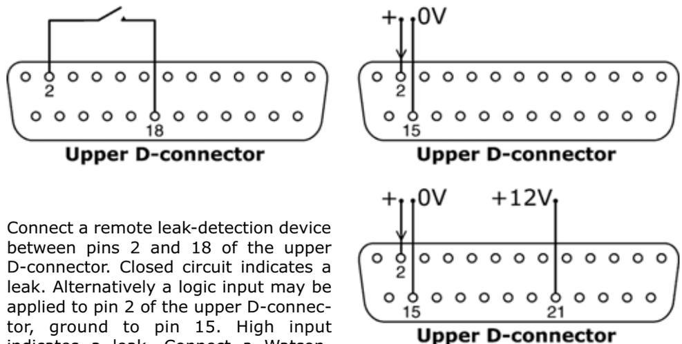
Connect a remote leak-detection device between pins 2 and 18 of the upper D-connector. Closed circuit indicates a leak. Alternatively a logic input may be applied to pin 2 of the upper D-connector, ground to pin 15. High input indicates a leak. Connect a Watson-Marlow leak detector in the same way, drawing 12V to power it from pin 21 of the upper D-connector.
