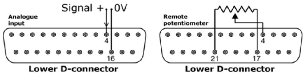
It is possible to control the speed of the pump remotely by one of these methods: a voltage analogue signal within the ranges 0-10V or 1-5V; or a current analogue signal within the range 4-20mA; or a remote potentiometer.
