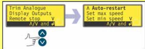
To move from one screen to subsequent screens, repeatedly press **DOWN**. Each item is highlighted in turn until the last item on the screen is highlighted.
