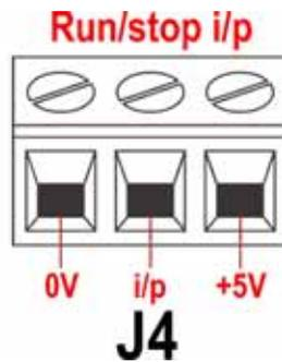
Remote run/stop: connect a remote switch between the **i/p** terminal and the **+5V** terminal of the Run/stop i/p connector (J4). Alternatively a logic input may be applied to the **i/p** terminal, ground to the **0V** terminal. High input stops the pump, low input runs the pump. With no connection or with the switch open, the pump will default to running. To change or set the sense of the run/stop input, see 16.5 *Remote stop* in the Setup menu.
