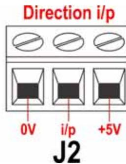
To enable remote direction control and disable the **DIRECTION (SHIFT, 1)** key on the keypad, link the terminals of the Direction enable link connector (J6). **Important: Apply no voltage whatever to the Direction enable link.** Connect a remote switch between the **+5V** terminal and the **i/p** terminal of the Direction i/p connector (J2). Open switch for clockwise rotation,
