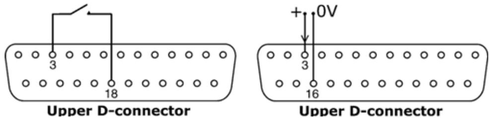
Connect a remote switch between pins 3 and 18 of the upper D-connector. Closed switch for automatic control; open switch for manual control. Alternatively a logic input may be applied to pin 3 of the upper D-connector, ground to pin 16. High input for automatic control; low input for manual control.
