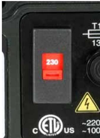
The voltage selector is mounted in the switchplate at the rear of the pump, protected from water by the 620N module (620DuN). The module must be removed to allow access to the switchplate. See 20.1 *620N module removal and replacement*. Set the voltage selector to 115V for 100-120V 50/60Hz supplies or 230V for 200-240V 50/60Hz supplies. Always check the voltage selector switch before connecting the mains supply. Make suitable connection to an earthed, single-phase mains electricity supply.
