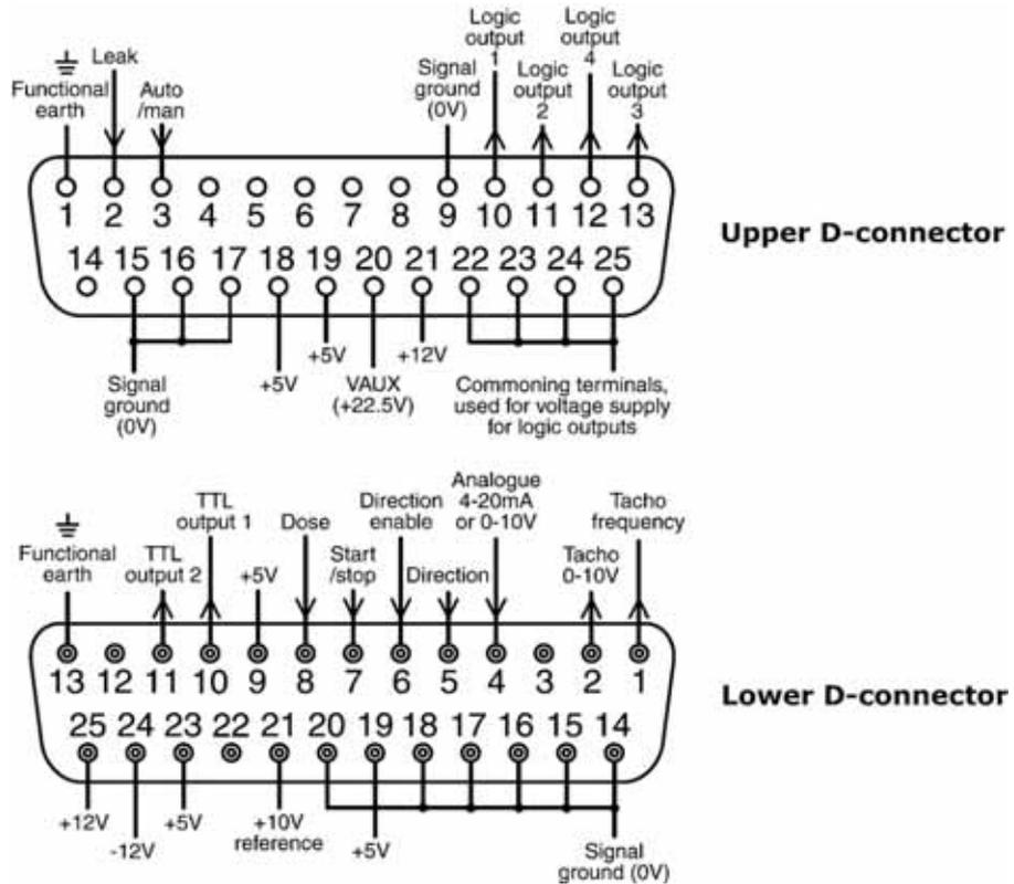
Recommended control cable: 7 strands 0.2mm, 24AWG, screened, circular, up to 25-core. The cable screen should be earthed either through the functional earth pin on the D-connector (pin 1 on the upper (male) 25-way D-connector) (pin 13 on the lower (female) 25-way D-connector), or through the metalwork of the socket or plug.
