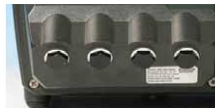
Recommended control cables must be used for the terminal blocks: metric = 0.14sq mm - 2.5sq mm solid and 0.14sq mm - 1.5sq mm stranded. USA = 26AWG - 14AWG solid and 26AWG - 16AWG stranded. Cable: circular. Max/min outside diameter to ensure a seal when passed through the standard gland: 9.5mm-5mm. **The cable section must be circular to ensure a seal.**
