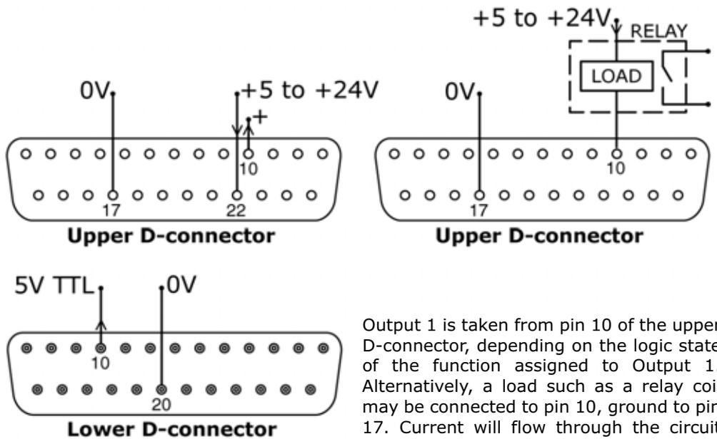
Output 1 is taken from pin 10 of the upper D-connector, depending on the logic state of the function assigned to Output 1. Alternatively, a load such as a relay coil may be connected to pin 10, ground to pin 17. Current will flow through the circuit depending on the logic state of the function assigned to Output 1. Do not connect to any device requiring more than 50mA.
