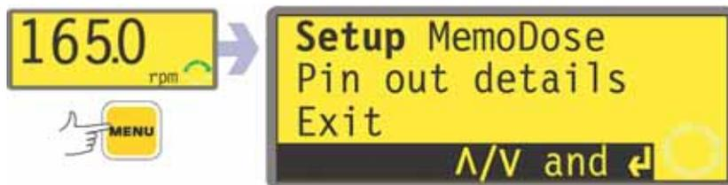
The main menu offers four options: **Setup**, **MemoDose**, **Pin out details**, and **Exit**. Use the **UP** and **DOWN** keys to make a choice. Press the **ENTER** key to confirm your decision.
