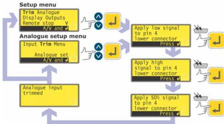
When the pump is under remote control, it tracks an analogue signal from the user's remote control system to pin 4 of the lower D-connector at the rear of the pump within the ranges 4-20mA, 0-10V or 1-5V. The **Trim** setup sequence allows the user to customise the process-signal-to-pump-speed calibration. The sequence may be entered directly from the Setup menu or from the Analogue setup menu.
