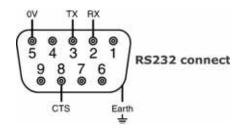
Recommended control cable: 7 strands 0.2mm, 24AWG, screened, circular, up to 4-core. The cable screen should be earthed through the metalwork of the shell.
