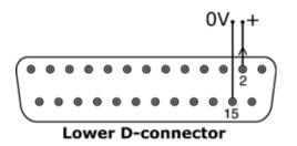
An analogue output signal is available as a 0V-10V signal on pin 2 of the lower D-connector. Ground to pin 15. The voltage is fixed and directly proportional to the pumphead rotation speed. 0V = zero speed; 10V = maximum speed.
