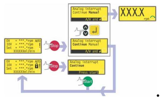
In an emergency press the  $\ensuremath{\text{STOP}}$  key. The pump stops and displays an interruption screen.
