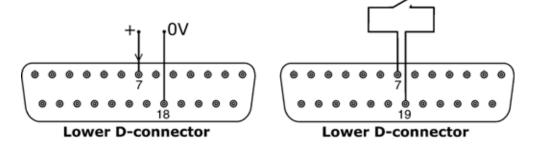
Remote run/stop: connect a remote switch between pins 7 and 19 of the lower Dconnector. Alternatively a logic input may be applied to pin 7 of the lower D-connector, ground to pin 18. High input stops the pump, low input runs the pump. With no connection or with the switch open, the pump will default to running. To change or set the sense of the run/stop input, see 18.11 Remote stop in the Setup menu.
