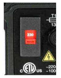
The voltage selector is mounted in the switchplate at the rear of the pump, protected from water by the 620N module (620DuN). The module must be removed to allow access to the switchplate. See 22.1 620N module removal and replacement. Set the voltage selector to 115V for 100-120V 50/60Hz supplies or 230V for 200-240V 50/60Hz supplies. Always check the voltage selector switch before connecting the mains supply. Make suitable connection to an earthed, single-phase mains electricity supply.
