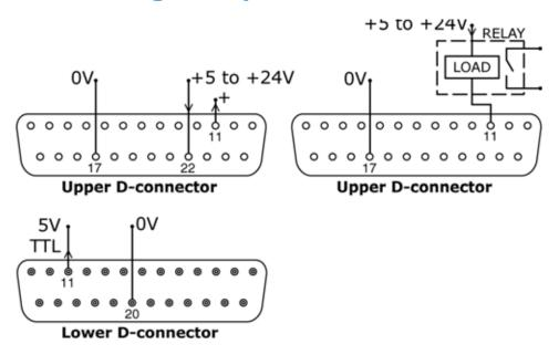
Output 2 is taken from pin 11 of the upper D-connector, depending on the logic state of the function assigned to Output 2. Alternatively, a load such as a relay coil may be connected to pin 11, ground to pin 17. Current will flow through the circuit depending on the logic state of the function assigned to Output 2. Do not connect to any device requiring more than 50mA.
