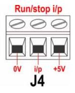
Remote run/stop: connect a remote switch between the i/p terminal and the +5V terminal of the Run/stop i/p connector (J4). Alternatively a logic input may be applied to the i/p terminal, ground to the 0V terminal. High input stops the pump, low input runs the pump. With no connection or with the switch open, the pump will default to running. To change or set the sense of the run/stop input, see 18.11 Remote stop in the Setup menu.
