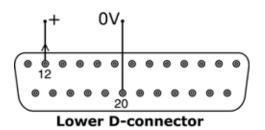
An analogue output signal is available as a 4-20mA signal on pin 12 of the lower Dconnector, requiring a  $250\Omega$  resister in series. Ground to pin 20. The current is fixed and directly proportional to the pumphead rotation speed. 4mA = zero speed; 20mA = maximum speed.
