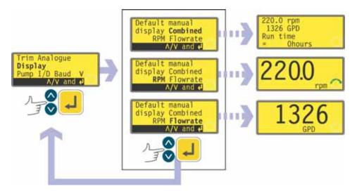
• In the first screen of the Setup menu select **Display** using the **UP** and **DOWN**
