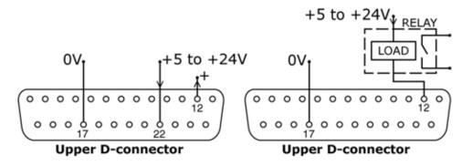
Output 4 is taken from pin 12 of the upper D-connector, depending on the logic state of the function assigned to Output 4. Alternatively, a load such as a relay coil may be connected to pin 12, ground to pin 17. Current will flow through the circuit depending on the logic state of the function assigned to Output 4. Do not connect to any device requiring more than 50mA.
