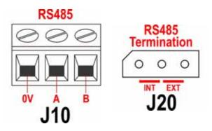
Connect your network link to J10 using a screened twisted pair: A to A, B to B, screen to 0V. Ensure that the pump is configured to operate under Network control. More than one pump may be controlled with the same RS485 signal: connect all pumps in parallel. See 22 Network control and operation.
