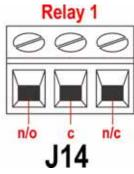
By default, Relay 1 is configured to indicate Run/Stop status; Relay 2 is configured to indicate Direction status; Relay 3 is configured to indicate Auto/man status; Relay 4 is configured
