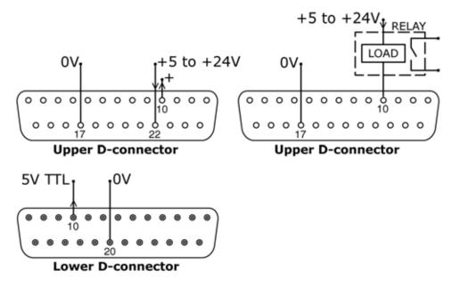
Output 1 is taken from pin 10 of the upper D-connector, depending on the logic state of the function assigned to Output 1. Alternatively, a load such as a relay coil may be connected to pin 10, ground to pin 17. Current will flow through the circuit depending on the logic state of the function assigned to Output 1. Do not connect to any device requiring more than 50mA.
