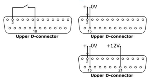
Connect a remote leak-detection device between pins 2 and 18 of the upper D-connector. Closed circuit indicates a leak. Alternatively a logic input may be applied to
