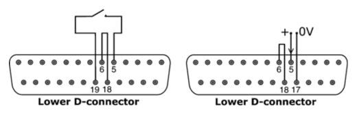
To enable remote direction control and disable the **DIRECTION (SHIFT, 1)** key on the keypad, link pins 6 and 18 of the lower D-connector. Connect a remote switch
