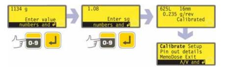
**Note**: If the pump has been set to display flow rate in units of mass (see 18.8 Flow units), as in this example, the pump displays a screen allowing you to confirm the specific gravity of the duty fluid immediately before the final press on **ENTER**.
