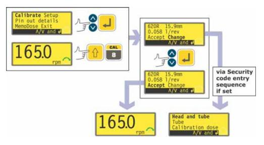
Use the UP and DOWN keys to highlight Calibrate in the main menu. Press ENTER to confirm.
