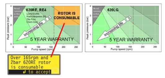
This pump's default running speed is 165rpm. It can be run at any speed up to 265rpm. Please note, however:
