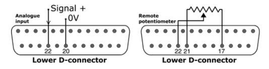
It is possible to scale the speed of the pump remotely by one of these methods: a voltage analogue signal within the ranges 0-10V or 1-5V; or a current analogue signal within the range 4-20mA; or a remote potentiometer.
