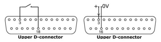
Connect a remote switch between pins 3 and 18 of the upper D-connector. Closed switch for automatic control; open switch for manual control. Alternatively a logic input may be applied to pin 3 of the upper D-connector, ground to pin 16. High input for automatic control; low input for manual control.
