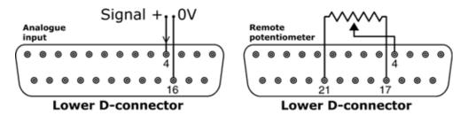
It is possible to control the speed of the pump remotely by one of these methods: a voltage analogue signal within the ranges 0-10V or 1-5V; or a current analogue signal within the range 4-20mA; or a remote potentiometer.
