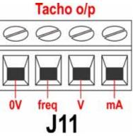
**Note**: If the mA output is to be used for reading from a multimeter, a  $250\Omega$  resistor is required in series.
