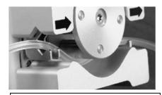
Ensure the tubing is correctly seated before closing the cover
