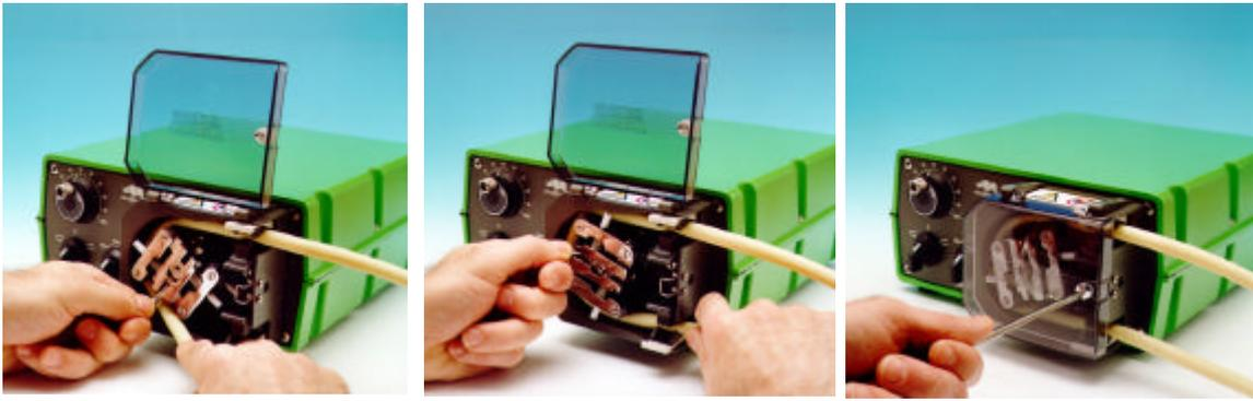
Fit the other end of the tubing into the second spring loaded clamp, ensuring that the tubing is not slack in the pumphead, since this can reduce tube life.
