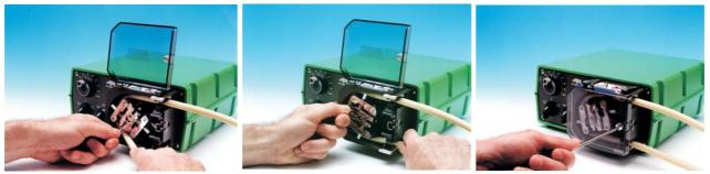
Fit the other end of the tubing into the second spring loaded clamp, ensuring that the tubing is not slack in the pumphead, since this can reduce tube life.
