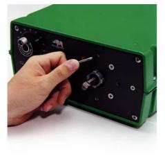
Fit the track in any one of three orientations, over the drive shaft and locating boss. Secure the track with the locating screw. Ensure the drive shaft is degreased before locating the rotor onto the shaft via the split collet. *Rotate the rotor until its guide rollers are aligned flush to the front edge of the track.* Tighten the rotor screw to a torque of 3Nm to prevent the collet slipping during operation.
