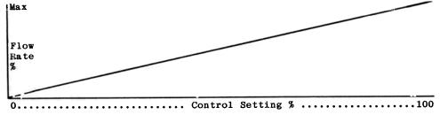
In addition, the 501U offers the facility of control of flow by virtually any of the process control signals in common use - for instance 0-10 mA as shown here:
