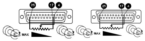
Note: As the remote potentiometer utilises the 0-10V range the speed response is only over  $^{10}/_{12}$ <sup>ths</sup> of the potentiometer's electrical travel. The signal overload illuminates at this point and there is no further increase in speed.
