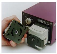
• Align the drive slot of the next pumphead to the drive tang of the extension pumphead, turn the next pumphead clockwise and snap into position.
