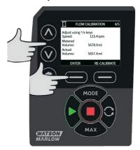
To accept the new calibration press **ACCEPT** or **RE-CALIBRATE** to repeat the procedure. Press **HOME** or **MODE** to abort.
