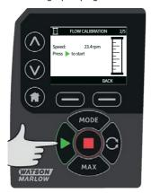
Press **STOP** to stop pumping fluid for the calibration.
