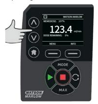
If **STOP** is pressed during dosing, the pump stops. Pressing **START** will resume, or discard, the interrupted dose depending on the settings in "Resume interrupted doses" on page 34.
