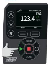
Starts the pump at the current flow displayed, and the display background changes to grey. If the pump is already running, pressing this has no effect.
