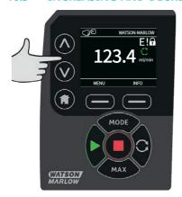
Using the  $\wedge$  and  $\vee$  keys will increase or decrease the flow rate.
