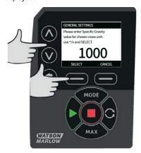
Use the  $\wedge$  / $\vee$  keys to enter the value of the specific gravity, and press **SELECT**.
