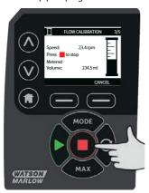
Use the  $\wedge$  / $\vee$  keys to enter the actual volume of fluid pumped.
