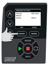
When MemoDose SETTINGS are complete the following screen is displayed; press **MEMODOSE** to start in MemoDose Mode or **BACK** to return to MemoDose settings.
