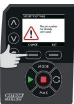
If the PIN entered does not allow access to the functionality the following screen will be displayed.
