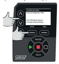
Now press  ${\bf CONFIRM}$  to verify that the number entered is the PIN you require. Press  ${\bf CHANGE}$  to return to PIN entry.
