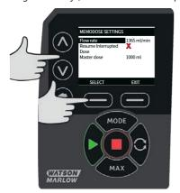
Using the  $\wedge$  / $\vee$  keys, enter the dose flow rate and press **SELECT**.
