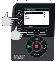
ENABLE user 1 security settings displays the PIN entry screen for User 1. To define a four digit User 1 PIN, use the  $\land / \lor$  keys to select each digit from 0-9. Once you have the required digit press the **NEXT DIGIT** key. After selecting the fourth digit press **ENTER**.
