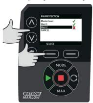
ENABLE user 2 security settings displays the PIN entry screen for User 2. To define a four digit User 2 PIN, use the  $\land / \lor$  keys to select each digit from 0-9. Once you have the required digit press the **NEXT DIGIT** key. After selecting the fourth digit press **ENTER**.
