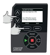
Now press  ${\bf CONFIRM}$  to check that the number entered is the PIN you require. Press  ${\bf CHANGE}$  to return to PIN entry.
