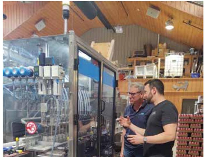
level, there is enough undulation to cause some turbulence of carbonated products, making them foam over continually, resulting in a cumulative loss of 4% of the product to the ground. The FaBLINE hoses, with their smooth, circular bore, have reduced this type of loss to 2.3%.
