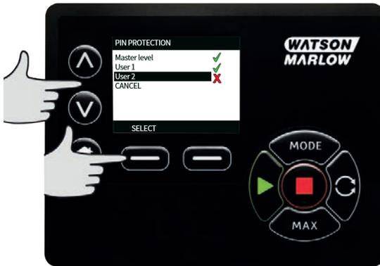
ENABLE user 2 security settings displays the PIN entry screen for User 2. To define a four digit User 2 PIN, use the  $\wedge$  /  $\vee$  keys to select each digit from 0-9. Once you have the required digit press the **NEXT DIGIT** key. After selecting the fourth digit press **ENTER**.
