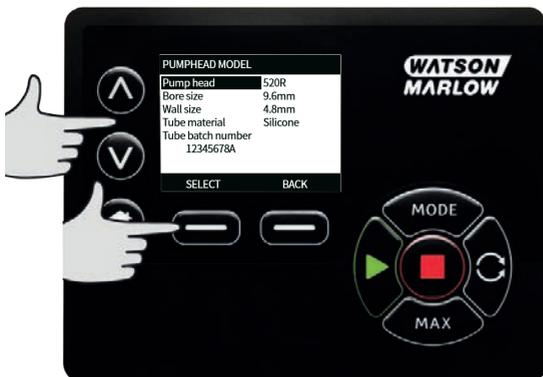
Use the  $\wedge$  /  $\vee$  keys to move the selection bar over the required pumphead type and press **SELECT**.
