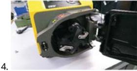
Ensure that the rotor hub spacer is still installed.
