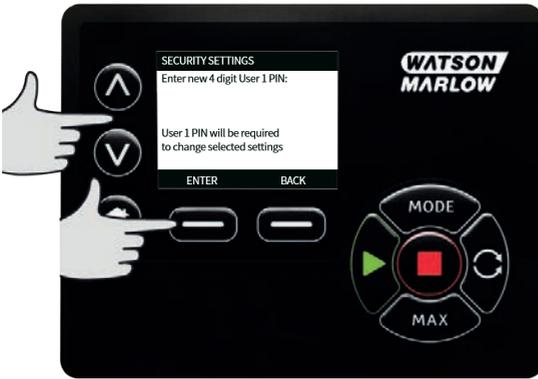
Now press **CONFIRM** to check that the number entered is the PIN you require. Press **CHANGE** to return to PIN entry.
