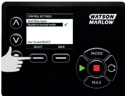
Use the ^ /v keys and press **SELECT** to choose the logic state of the chosen input for your connected control hardware.
