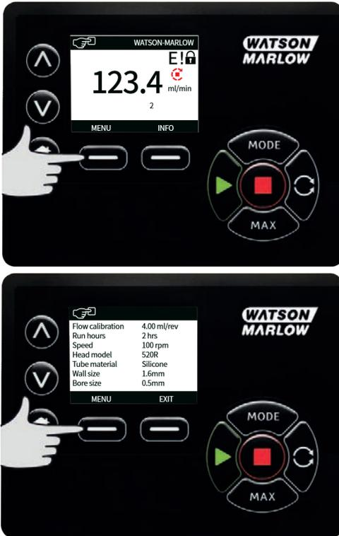
This will display the main menu as shown below. Use the  $\wedge$  /  $\vee$  keys to move the selection bar between the available options.
