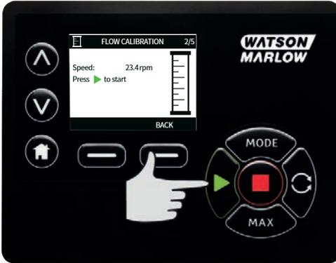
Press **STOP** to stop pumping fluid for the calibration.
