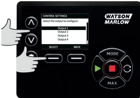
Use the  $\wedge$  /  $\vee$  keys and press **SELECT** to choose which pump status you require for the chosen output. The tick symbol indicates the current setting.
