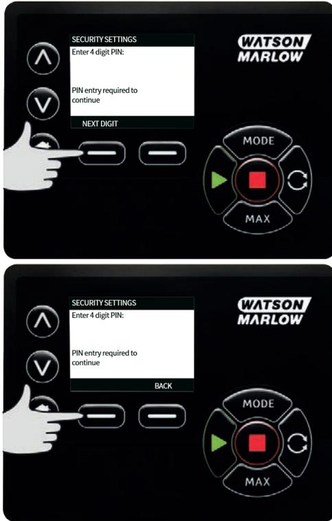
If an incorrect PIN has been entered the following screen will be displayed. NOTE: this screen will also display if the PIN entered does not allow access to that functionality.
