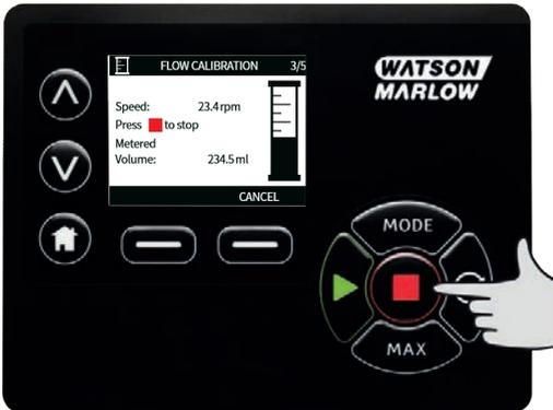
Use the  $\wedge$  /  $\vee$  keys to enter the actual volume of fluid pumped.
