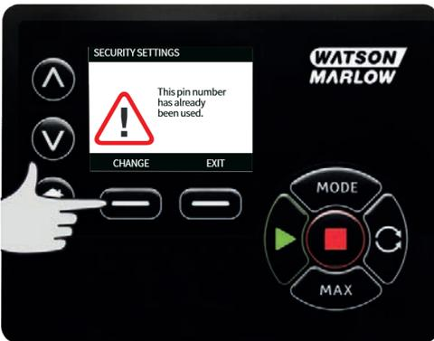
If the PIN entered does not allow access to the functionality the following screen will be displayed.
