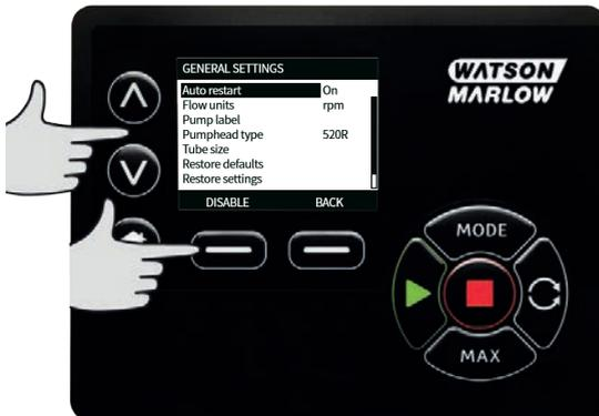
Use the  $\wedge$  /  $\vee$  keys to move the selection bar over **Pumphead** and press **SELECT**.
