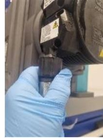
Ensure that any bend radius of the hose exceeds the 76 mm (3") minimum requirement.
