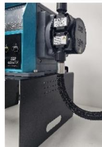
7. Check the full length and routing of the hose to be sure there are no twists, kinks or rubbing of the hose against itself (for example when looped) or against another surface (for example: the edge of the access hole or a shelf).
