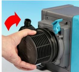
To disengage the pumphead from the drive, rotate it in a clockwise direction by approximately 15°.
