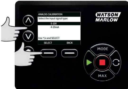
The pump gives the option to enter the high and low mA or V signals manually or via the analog input. Entering mA values is described here and the process for entering Voltage signals is identical.
