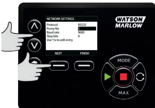
Note: If the network protocol is RS485 the maximum number that can be assigned to the pump is 32, otherwise it is 16.
