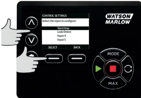
The default is ✖. The start/stop input is not disabled in manual mode. Press **SELECT** to change the setting to ✔.
