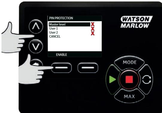
ENABLE user 1 security settings displays the PIN entry screen for User 1. To define a four digit User 1 PIN, use the  $\wedge$  /  $\vee$  keys to select each digit from 0-9. Once you have the required digit press the **NEXT DIGIT** key. After selecting the fourth digit press **ENTER**.
