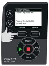
The following screen will be displayed to indicate that the Master PIN has been applied to access all functionality. Press **NEXT** to selectively enable functionality access for User 1 and User 2.
