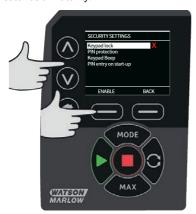
Once locked it will display the screen below when any key is pressed. To unlock the keypad press the two **UNLOCK** keys together.
