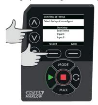
The default is  $\times$ . The start/stop input is not disabled in manual mode. Press **SELECT** to change the setting to  $\checkmark$ .
