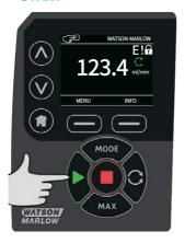
Starts the pump at the current flow displayed, and the display background changes to grey. If the pump is already running, pressing this has no effect.
