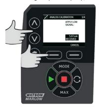
ACCEPT appears when low mA signal is within tolerance limits. Press **ACCEPT** to accept the low signal input or **CANCEL** to return to the previous screen.
