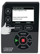
To define the allowed functionality, use the  $\land \land \lor$  keys to select the functionality and press **ENABLE**. User 1 PIN will allow access to only the enabled functionality, to disable functionality, highlight the enabled functionality and press **PISABLE**. When all the required functionality has been enabled, press **FINISH**.
