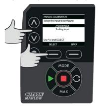
Select the input signal type using the  $\land / \lor$  keys and press **SELECT**.
