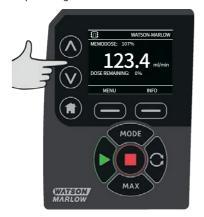
If **STOP** is pressed during dosing, the pump stops. Pressing **START** will resume, or discard, the interrupted dose depending on the settings in "Resume interrupted doses" on page 83.
