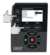
Note: If the network protocol is RS485 the maximum number that can be assigned to the pump is 32, otherwise it is 16.
