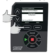
Select the input signal type, using the  $\land$  /  $\lor$  keys, and press **SELECT**.
