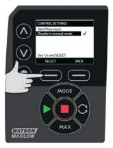
Use the  $\land$   $\land$  keys and press **SELECT** to choose the logic state of the chosen input for your connected control hardware.
