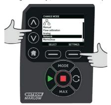
In both RS485 and RS232 mode there is the option to run in ENHANCED or BASIC communication protocol.
