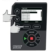
If a LoadSure element has been selected then the tube size is displayed as pressure and bore.
